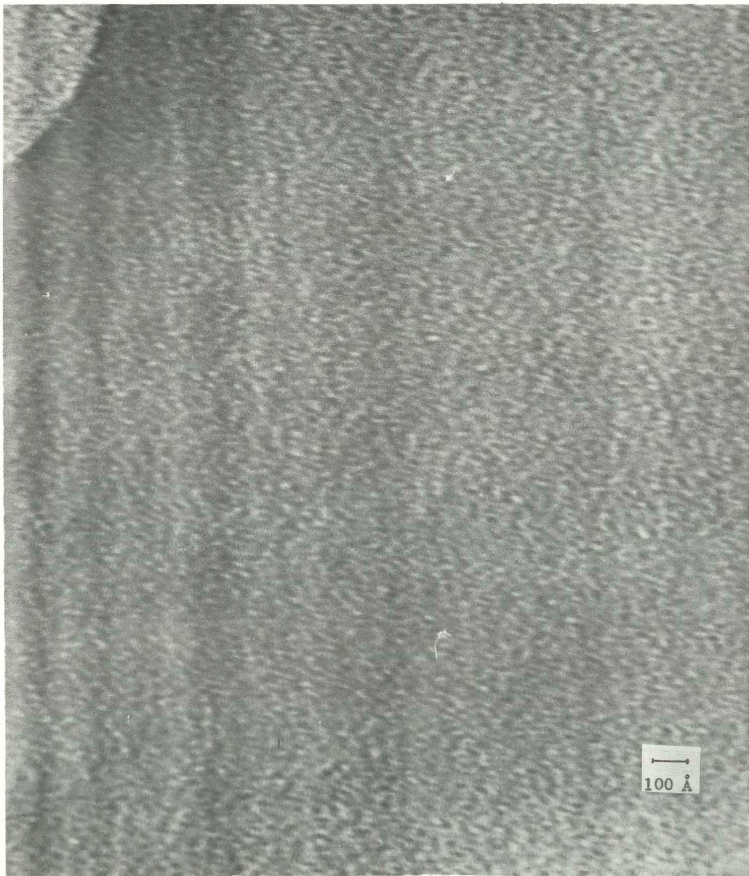
Fig. 10 Synthoil Crude Asphaltene Evaporated Carbon Support Film (910,000x).
