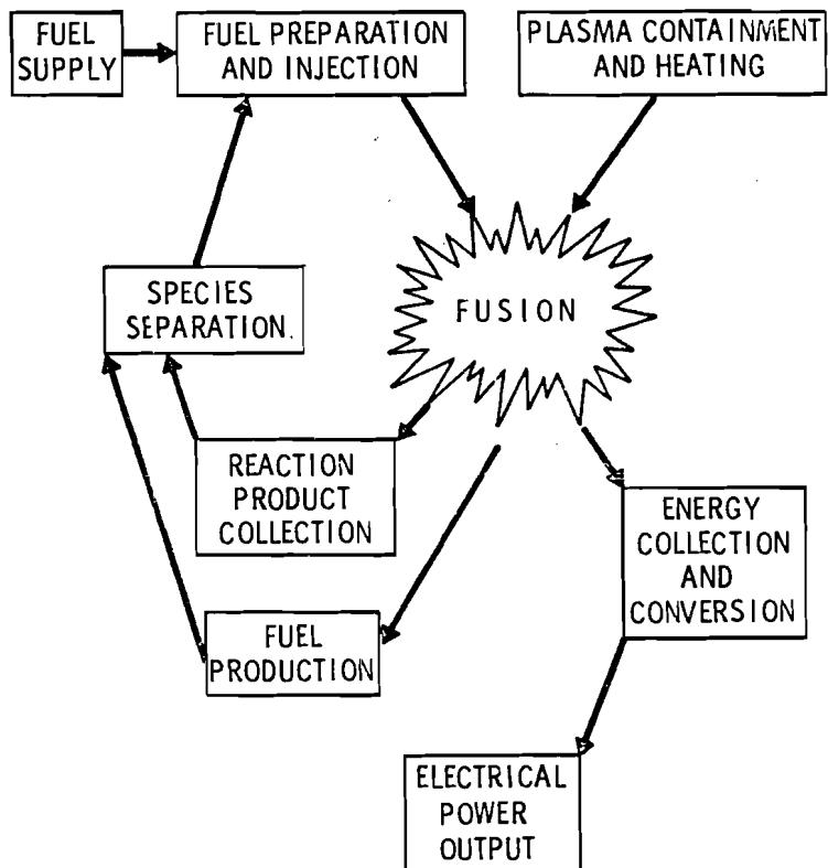
FIGURE 1. Functional Components of CTR Power Plant Systems
