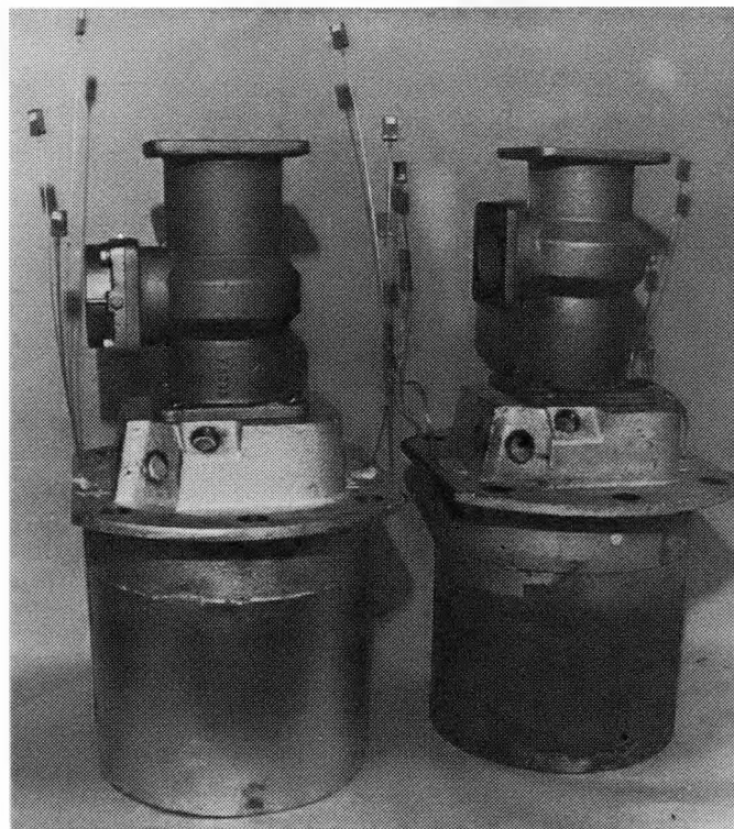
Figure 5.3-15. Original and Upgraded Reformer Burners
