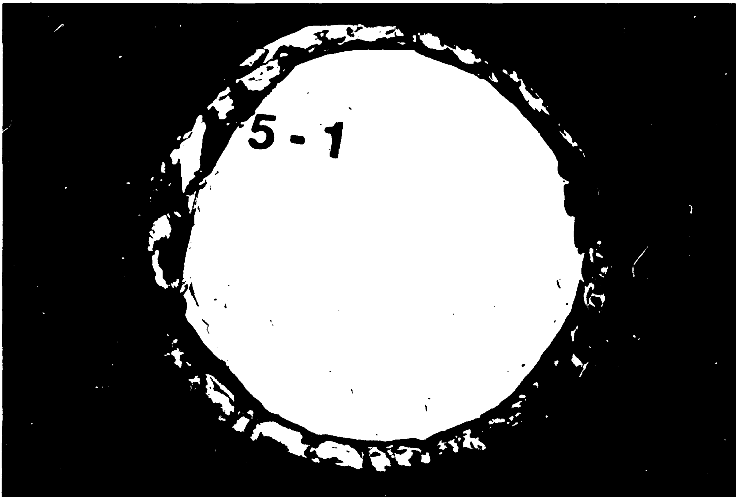
Fig. 20. Combination 5-1 neat-resin sample after cryogenic shock/soak
