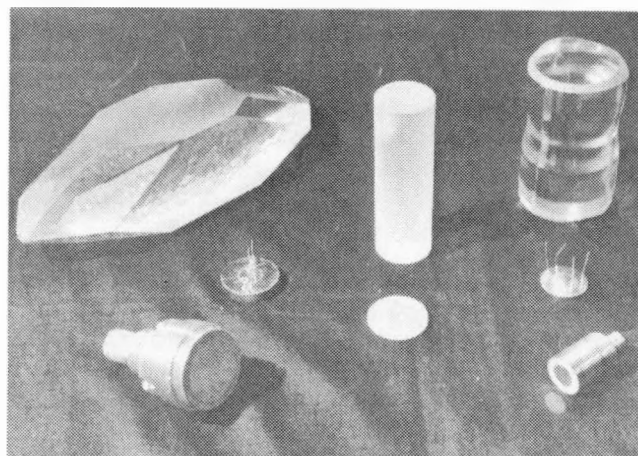
Figure 7. Crystals and stress gauges (left-to-right) of quartz, sapphire and lithium niobate
