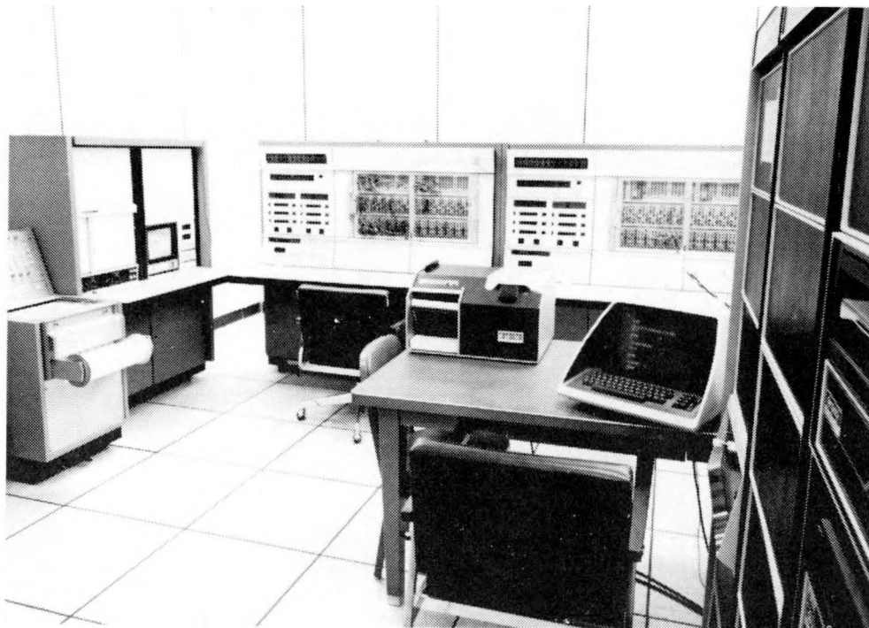
Figure 2. The AD/FIVE-PDP 11/45 hybrid computer
