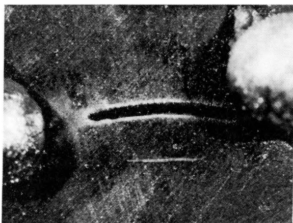
Figure 1. Current filament formed on surface of AsTeI semiconducting glass during electrical switching
