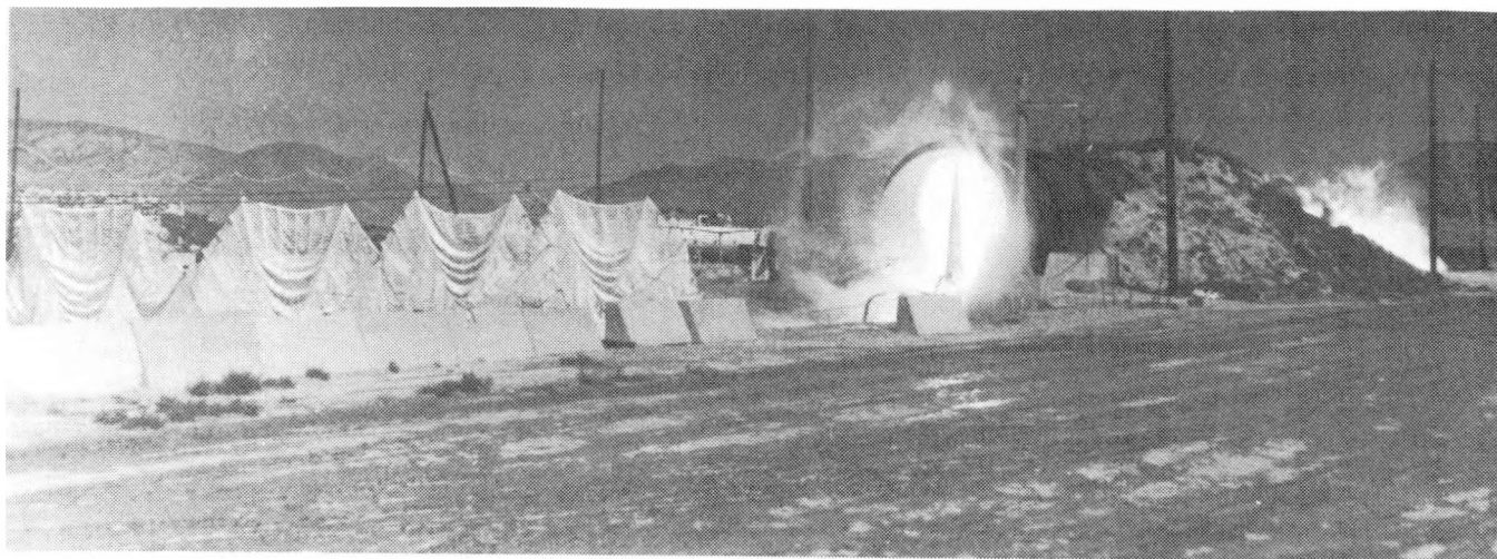
Figure 4. Blast testing of a missile system in a shock tube
