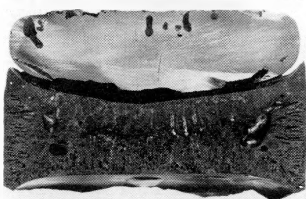
Figure 2. Cross section of special nuclear material that has been chemically altered into slag and metallic components, both of which contain uranium, but in dilute, unusable form.
