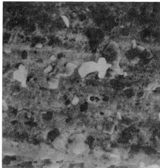
Figure 2. Corrosion on Tophet C after exposure to potassium hexacyanocobaltate for 260 days at 50 percent humidity. Scanning electron micrograph at 3000X.
