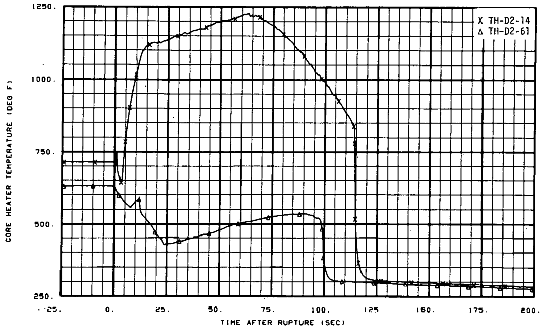
Fig. 81 Core heater temperature, Rod D-2 (TH-D2-14, TH-D2-61), from -24 to 200 seconds.
