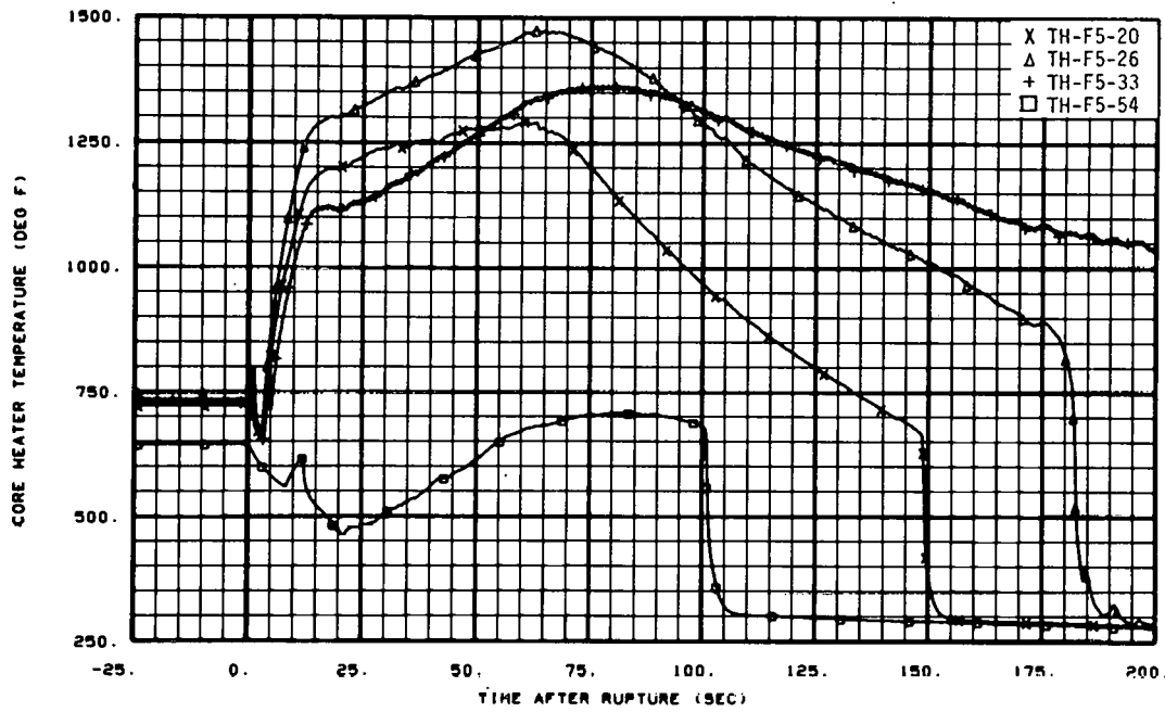
Fig. 109 Core heater temperature, Rod F-5 (TH-F5-20, TH-F5-26, TH-F5-33, TH-F5-54), from -24 to 200 seconds.
