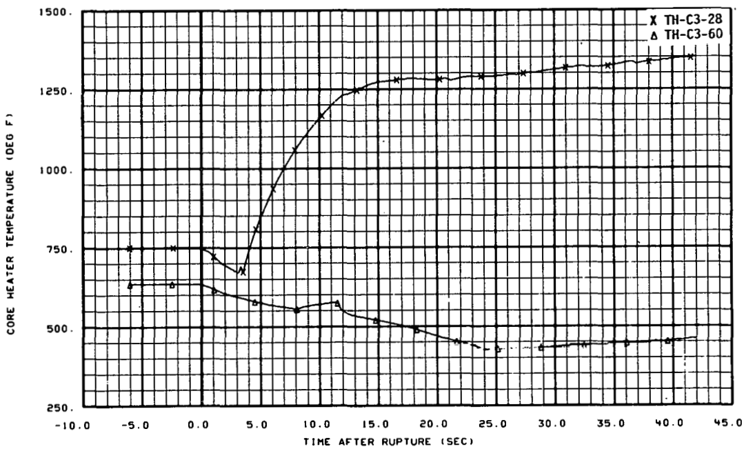
Fig. 70 Core heater temperature, Rod C-3 (TH-C3-28, TH-C3-60), from -6 to 42 seconds.
