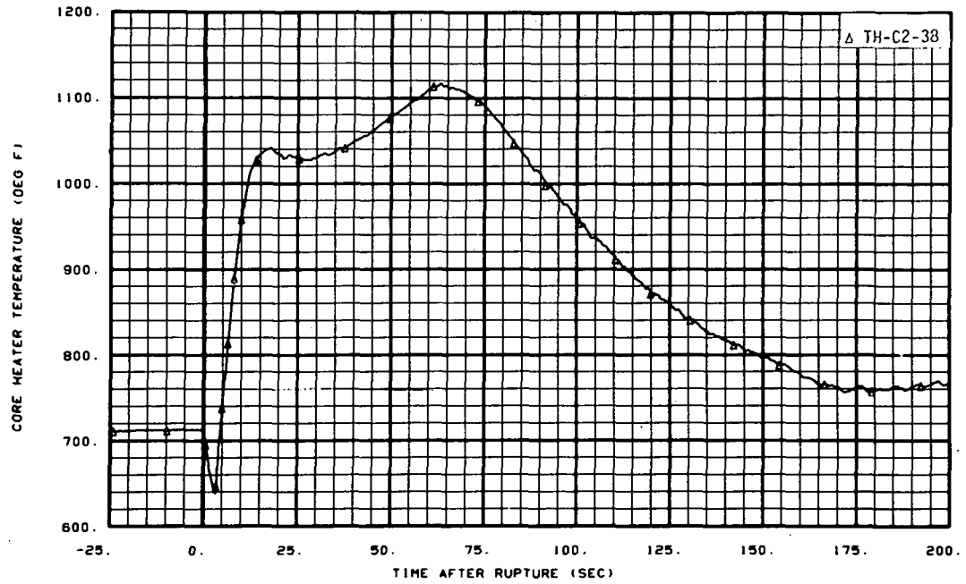
Fig. 67 Core heater temperature, Rod C-2 (TH-C2-38), from -24 to 200 seconds.
