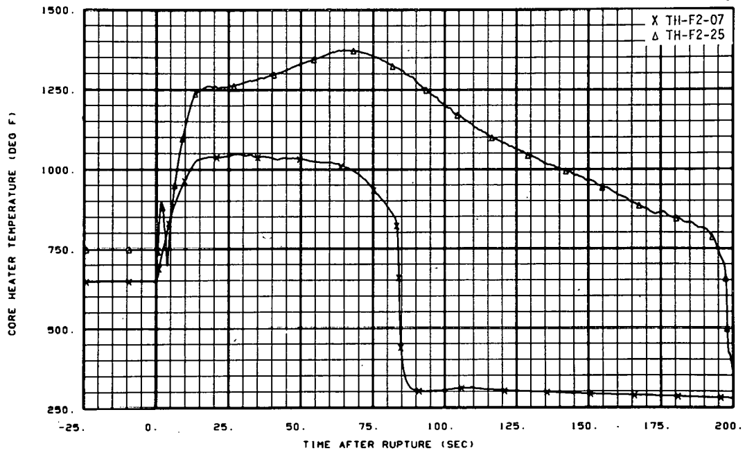
Fig. 103 Core heater temperature, Rod F-2 (TH-F2-07, TH-F2-25), from -24 to 200 seconds.
