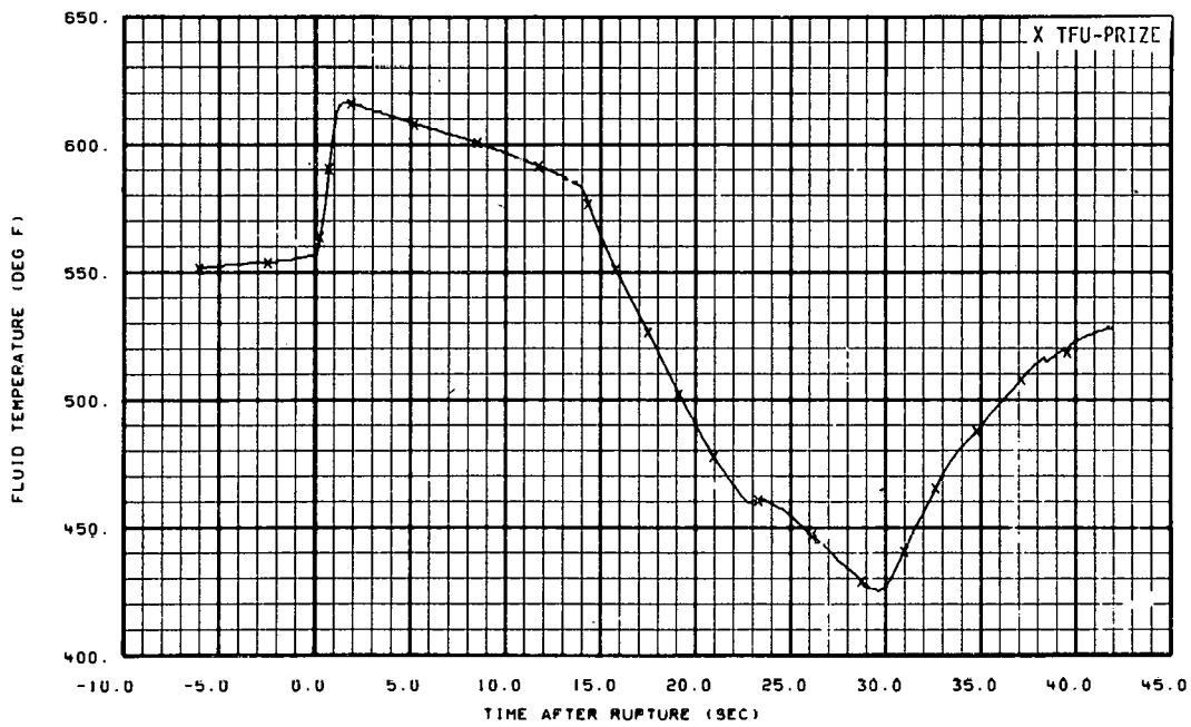
Fig. 38 Fluid temperature in pressurizer surge line (TFU-PRIZE), from -6 to 42 seconds.
