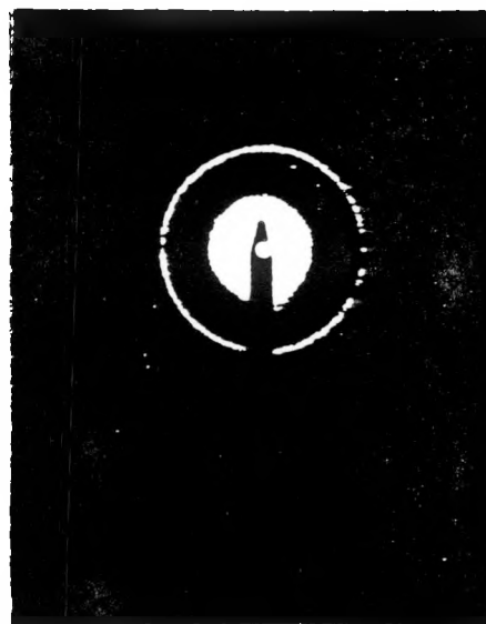
Figure 2: TEM electron diffraction pattern for TiN deposited at 200 °C.
