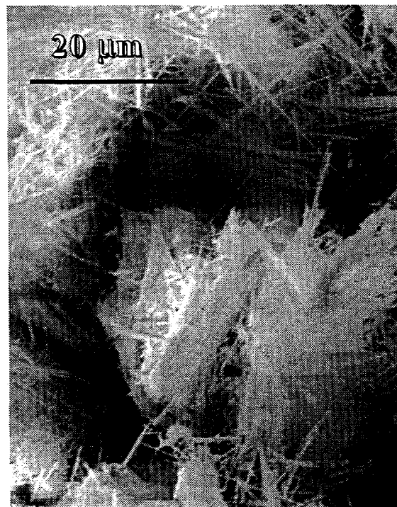
Figure 3. Scanning electron micrograph of the Zr-phase.
