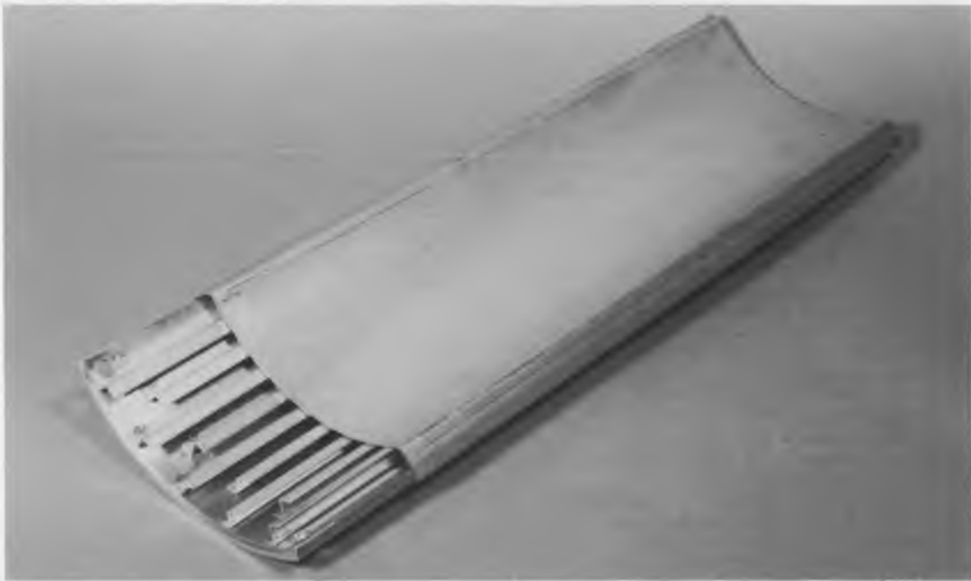
Figure F-2. Photograph of the inner and outer shell of one calorimeter quadrant, with the inner shell slid back to reveal the water-flow baffles.
