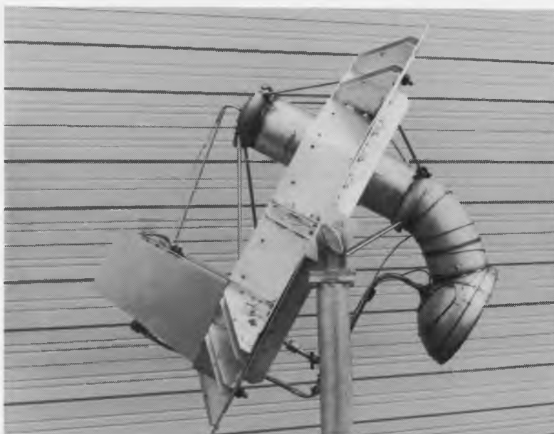
Figure B-9. Photograph showing a side view of the pool-boiler receiver in the mounting ring.
