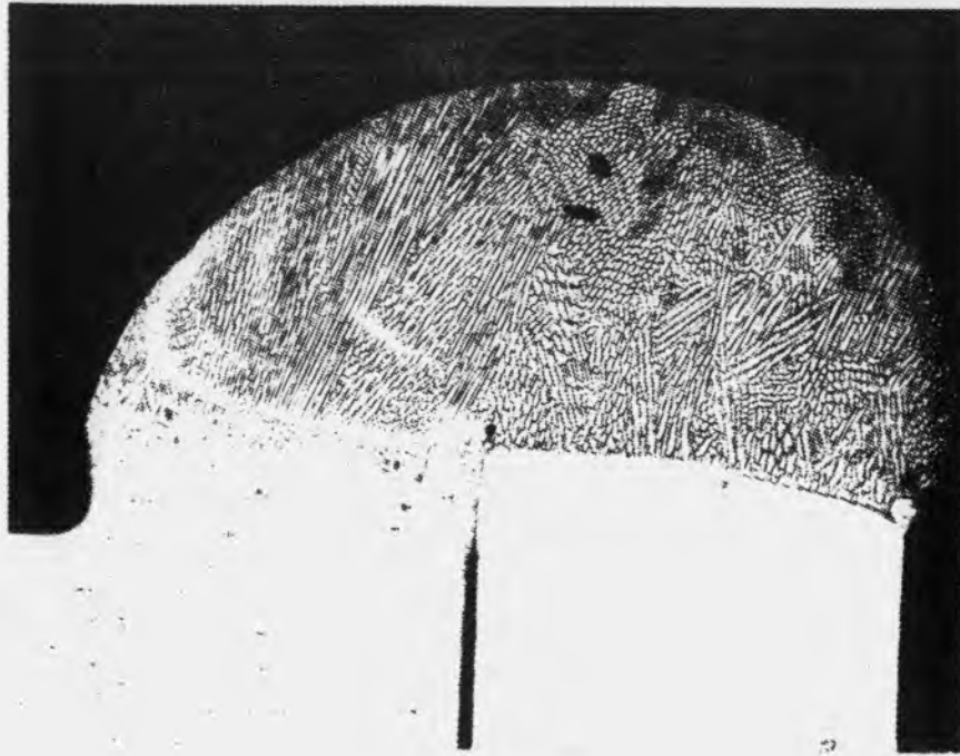
Figure 1. Cross section of Haynes 230/Inconel 600 weld in standing edge configuration. 100X magnification.
