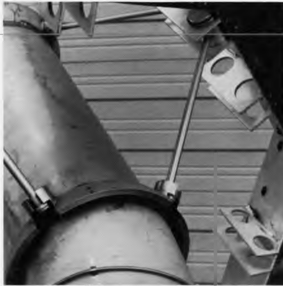
Figure B-6. Photograph showing the spoke attachments to the pool-boiler hub assembly.
