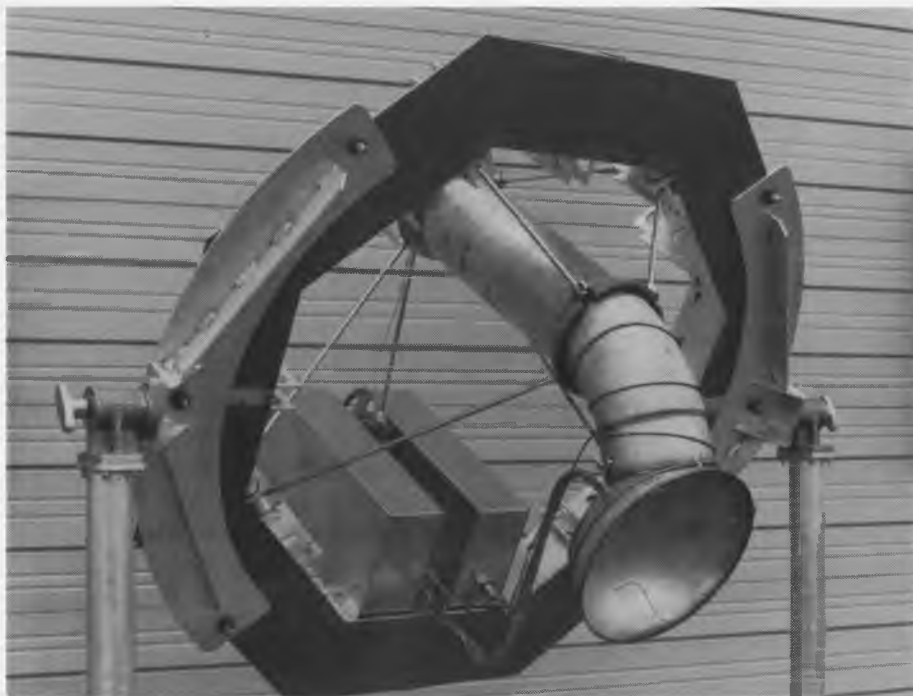
Figure B-5. Photograph of the pool-boiler receiver in the mounting ring.
