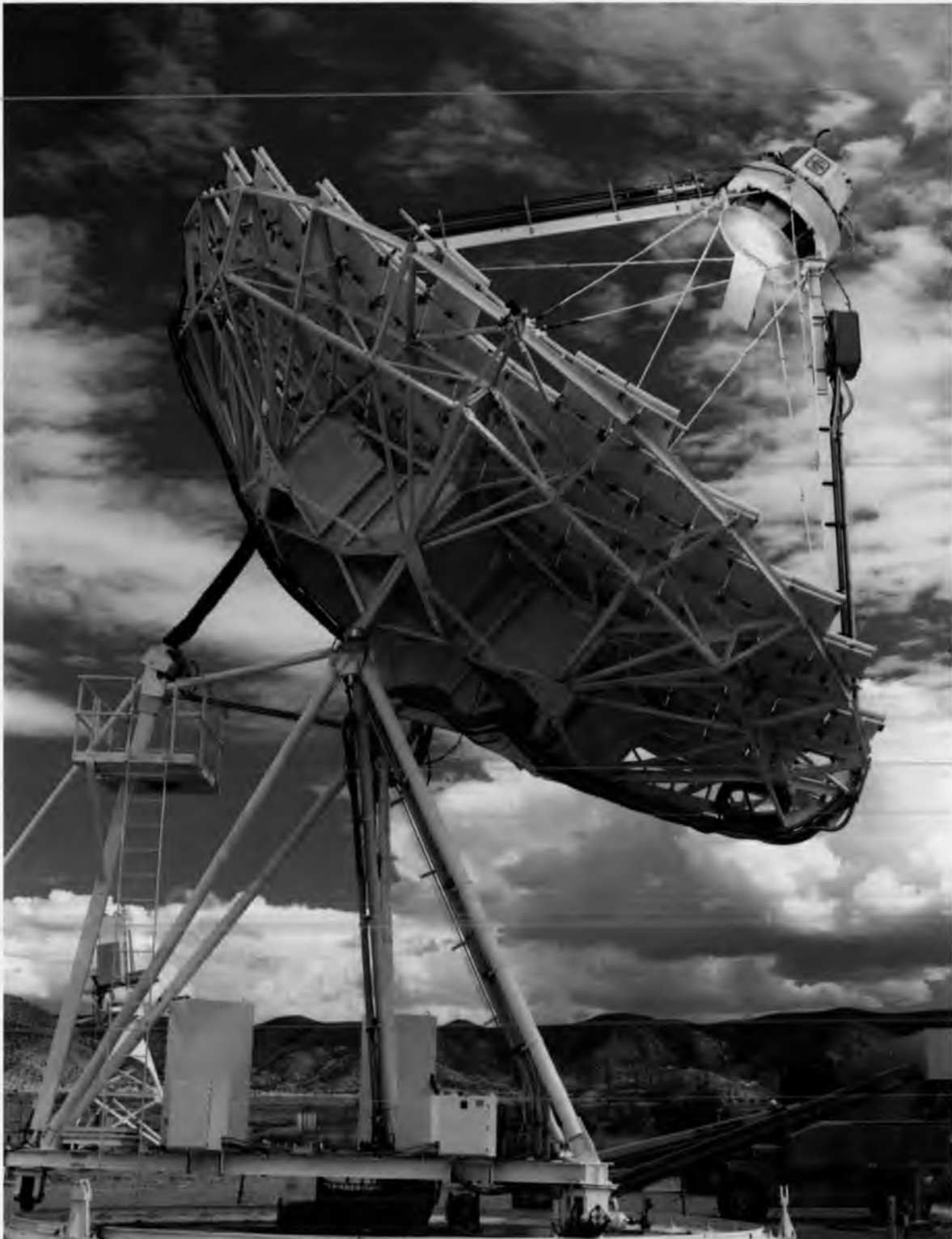
Figure 5. The Sandia reflux pool-boiler receiver during the on-sun testing.
