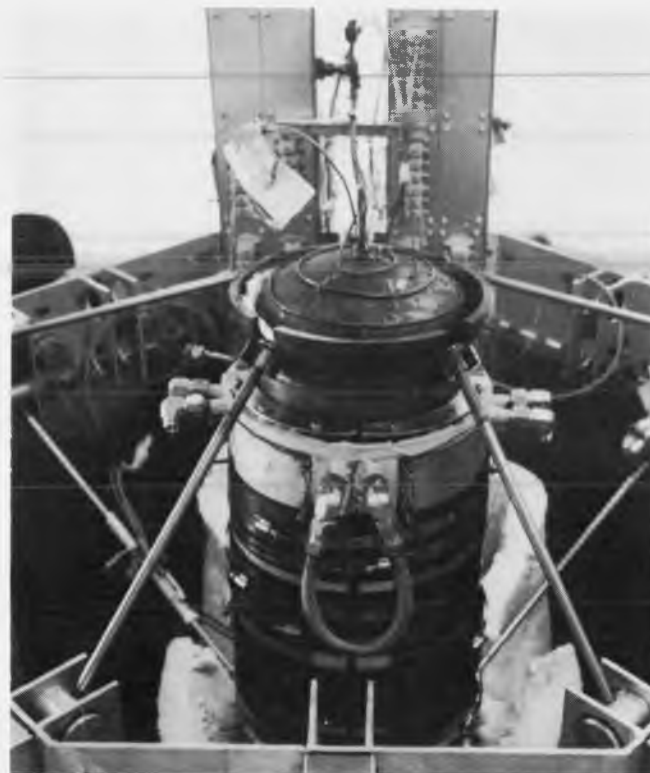
Figure F-5. Photograph of the four calorimeter quadrants installed on the pool-boiler receiver with one water connection between quadrants completed.
