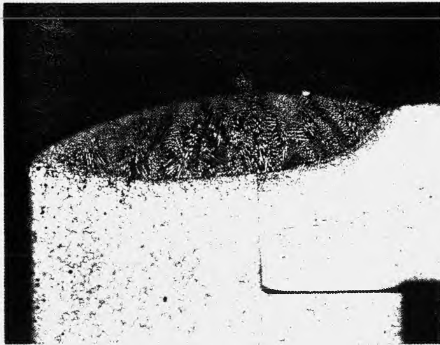
Figure 1. Cross section of autogenous Haynes 230 corner groove weld (no filler metal). 32X magnification.
