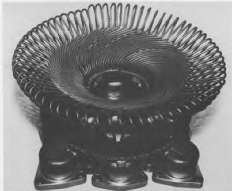
Figure 2. United Stirling of Sweden heater head used on the Advanco dish-Stirling Module. The heater head tubes were expanded to make the solar flux levels lower and more uniform.
