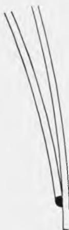
Figure 1. Illustration of slight change needed to make the rim weld inspectable (compare with Figure 2 "Current Rim Design").
