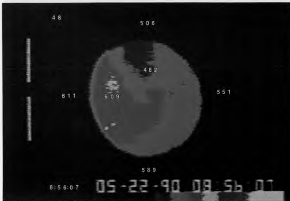
Figure P-3. Infrared video image taken 15 seconds after startup. The high flux inner ring predicted by CIRCE2 appears to be offset to the left indicating a 3 milliradian concentrator mistrack. The image is a reversed left-to-right (by the mirror) view of what an observer, standing at the concentrator and looking at the receiver, sees.
