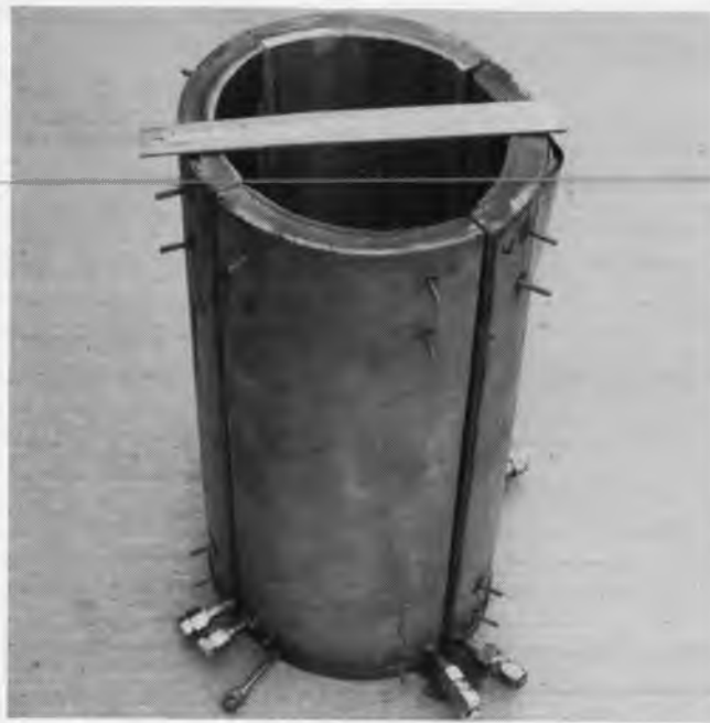
Figure F-4. Photograph of the four calorimeter quadrants grouped as installed on the pool-boiler receiver. The large and small fittings at the bottom are the water and gas ports, respectively.
