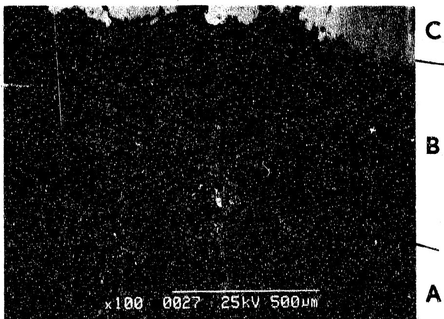
Figure 68. Cu depleted layer next to the CEROX coating (Anode 13614-53, 100X). C=CEROX, B=Cu depleted zone, A=Cu oxide region
