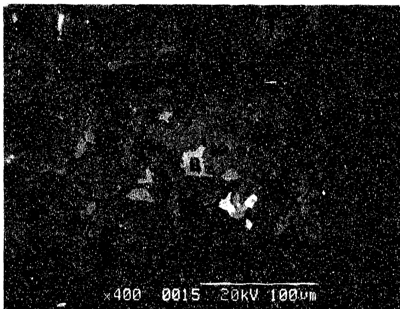
Figure 80. The porous zone from Figure 78 contains primarily NiO (B) and \text{NiFe}_2\text{O}_4 (A) (Anode 13614-21, 400X).
