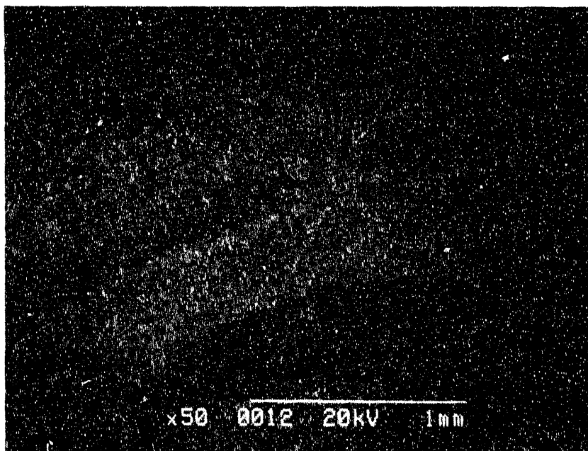
Figure 77. Porous and dense bands alternate within the oxidized region (Anode 13614-21, 50X).
