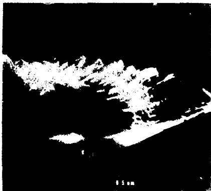
Fig. 2. Dark field electron micrograph of a broken fragment of silicon carbide showing a number of partially healed, secondary cracks stemming from the serrated fracture edge. (XBB 754-3148)
