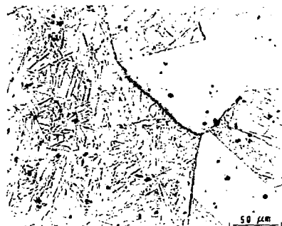
Fig. 1. Optical micrograph showing the "ghost-like" substructure after the ausaged and LN 2 -cooled specimen is reverted to austenite. (XBB 759-6731)
