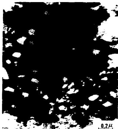
Fig. 2. Transmission electron micrograph. Maraged (550°C/5 hr/Air Cool), rapidly reverted to austenite in a salt bath (750°C/2.5 min.), and transformed to martensite by cooling to room temperature.
