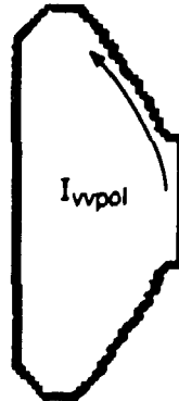
Fig. 1. Poloidal current flow in a tokamak vacuum vessel.
