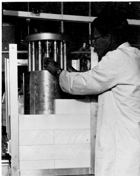
Fig. 37. The ^{15}\text{He} tubes supported by the high-voltage distribution junction box are being lowered into the moderator. The cadmium liner about the moderator and the partially stacked polyethylene shield are also shown.
