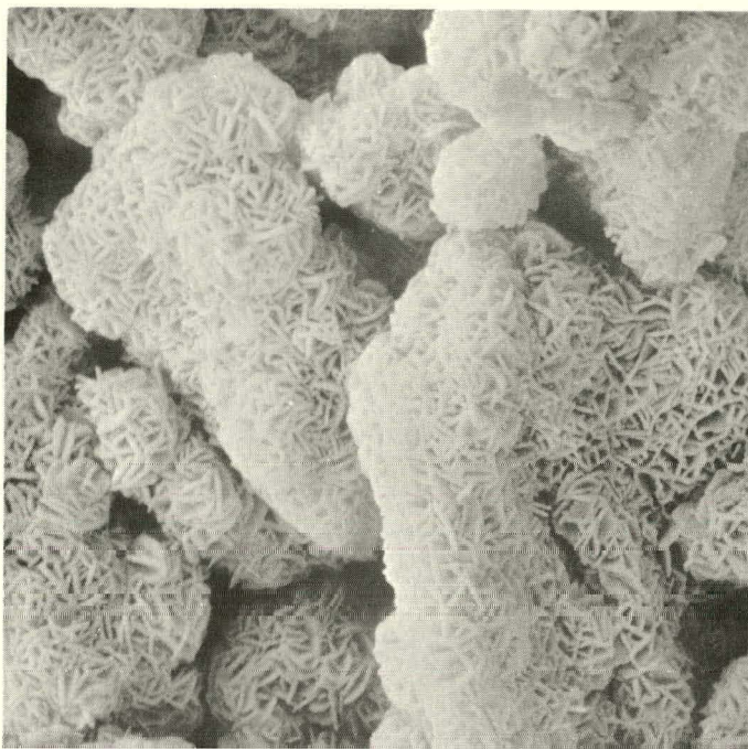
Fig. IV-3. Yttria Powder Treated with 3M Nitric Acid and Sintered at 1100°C (6000X)
