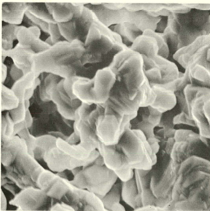
Fig. IV-4. Yttria Powder Treated with 3M Nitric Acid and Sintered at 1350°C (6000X)
