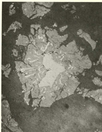
STAGE II. Inner Region--FeS; Intermediate Region-- \text{Li}_2\text{FeS}_2 , Fe; Outer Region--J.
