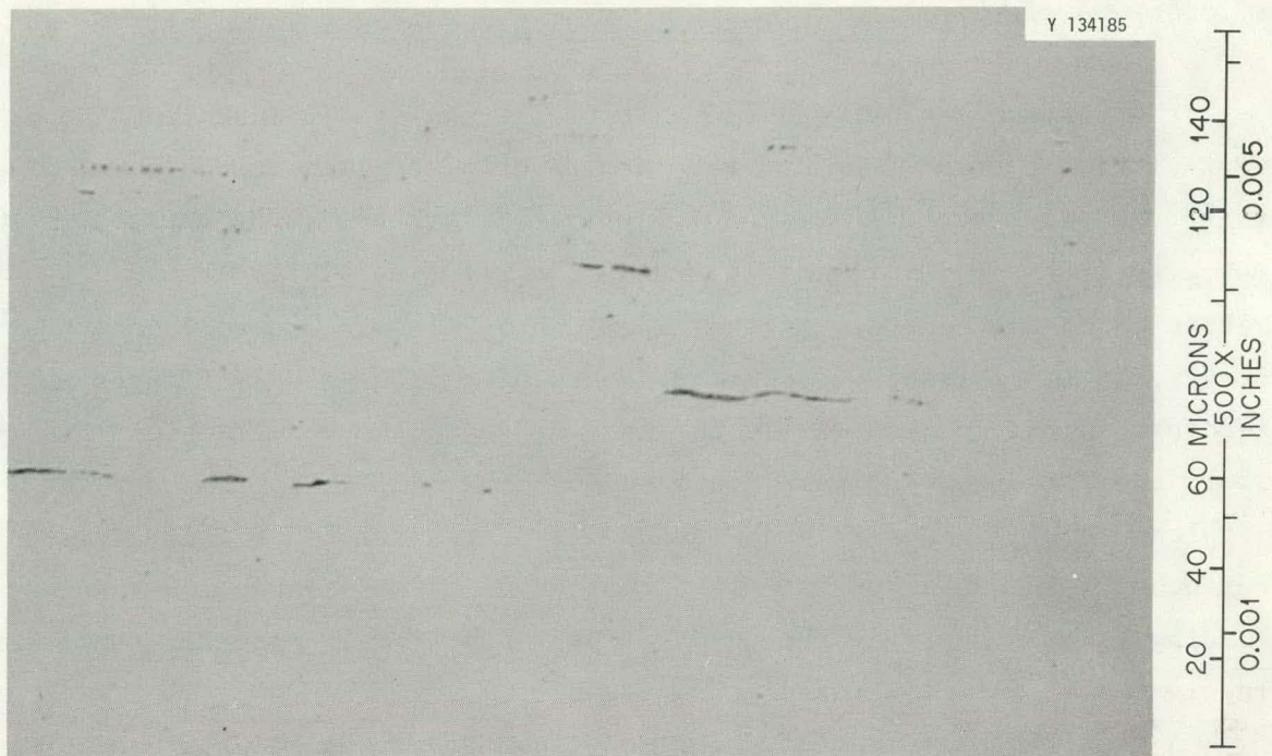
Fig. 7.16. Photomicrograph showing sulfide stringers in the interior of a randomly selected section of circumferential tendons employed in the thermal cylinder test (500x). (Original reduced 43%)
