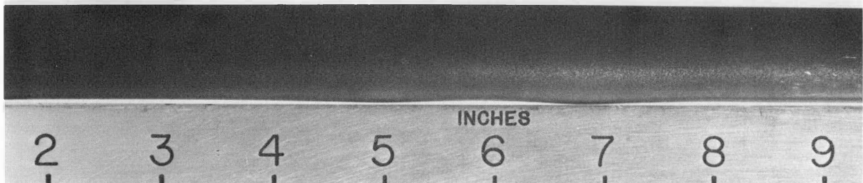
Haynes 188 tube ballooning 1037°C (1,900°F)
