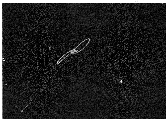
Figure B-1 POOLSIDE EDDY CURRENT DATA FOR ROD JBP-027 FROM B-042 SHOWING SIGNALS AT 53 1/4 AND 59 5/16 INCHES FROM THE BOTTOM OF THE ROD. (TOP - RECORDER TRACES, BOTTOM - CORRESPONDING OSCILLOSCOPE SIGNATURES)
