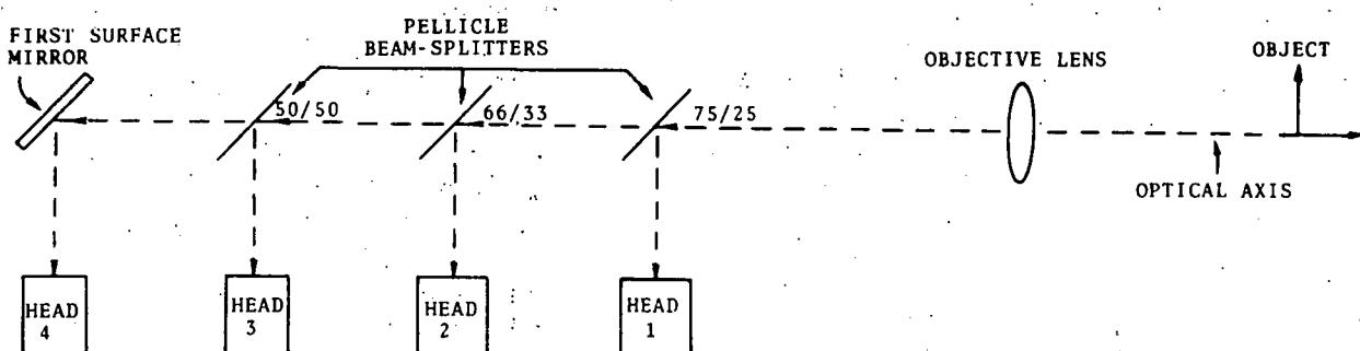
Fig. 1. Optical Arrangement of Marco M4 Camera
