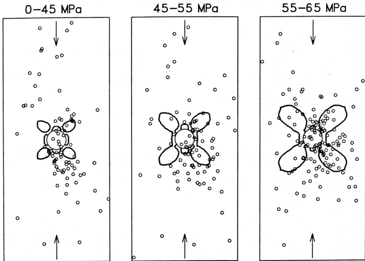
Figure 2. Locations for AE events occurring at stresses between (a) 0 and 45 MPa, (b) 45 and 55 MPa and (c) 55 and 65 MPa. A circle is plotted at each event location with the size of the circle corresponding to the location uncertainty as judged by the magnitude of the time residuals. Solid contours are the boundary of the zone where damage has occurred between the start and end of each step. Uniaxial load was applied along the axis indicated by the arrows.
