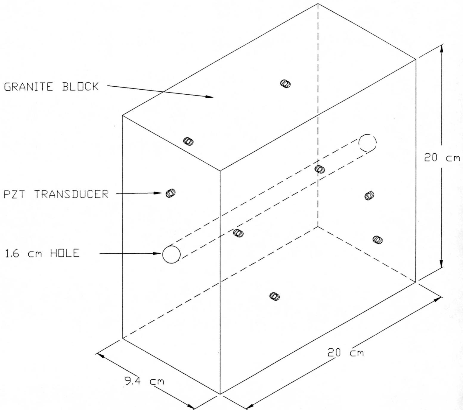
Figure 1. Diagram of sample showing transducer and strain gage locations.
