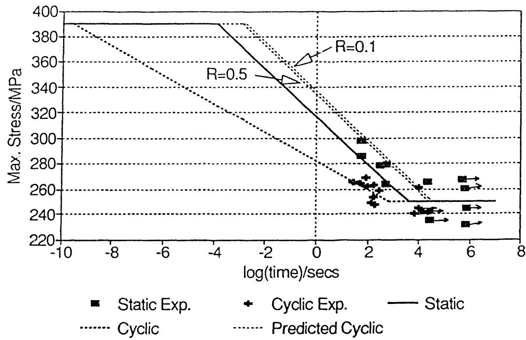
Fig. 2: Stress/life data for MS-grade Mg-PSZ ( $K_c \approx 11.5 \text{ MPa}/\text{m}$ ) under quasi-static and cyclic ( $R = 0.1$  and  $0.5$ ) loading, showing a comparison of experimental vs. predicted lifetimes [18].
