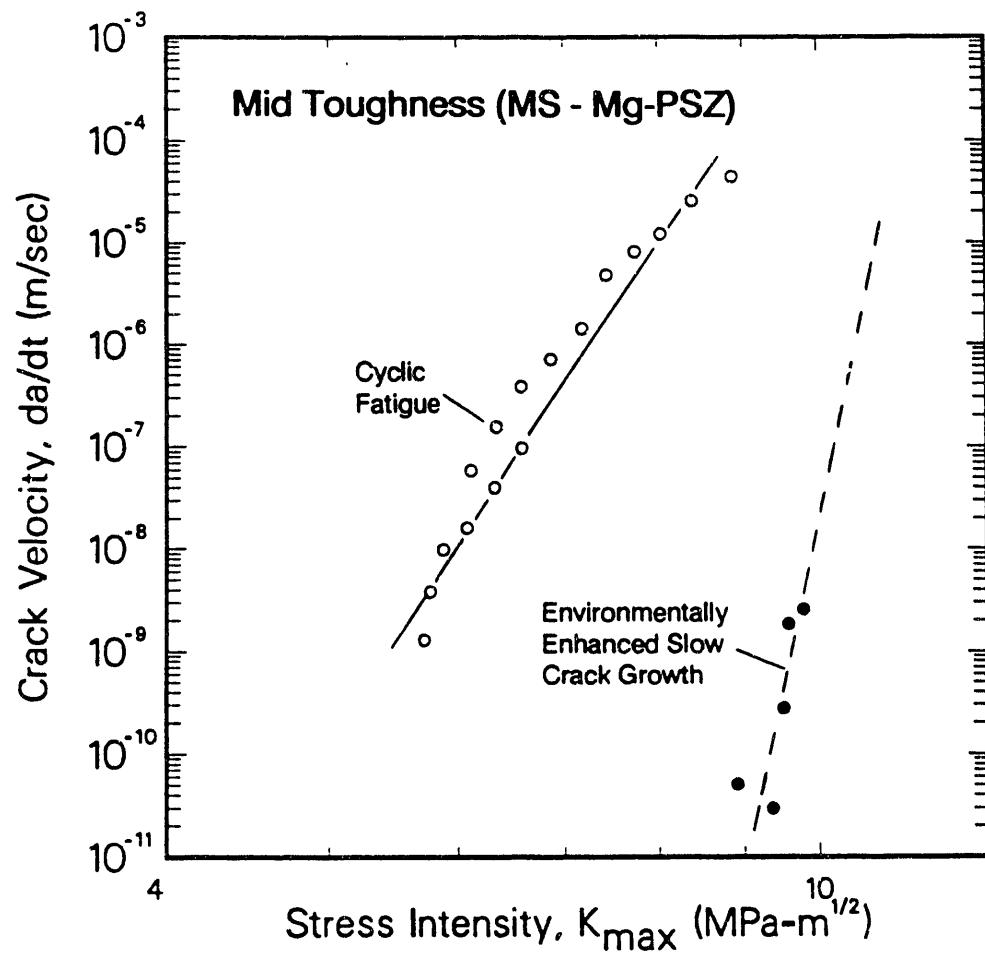
Fig. 4: Comparison of the crack velocity vs. maximum stress intensity ( $K_{max}$ ) curves for static fatigue (slow crack growth) and cyclic fatigue ( $R = 0.1$ ) in MS-grade Mg-PSZ in a moist air environment, showing cyclic crack velocities up to 7 orders of magnitude faster at equivalent  $K_{max}$  levels [7].
