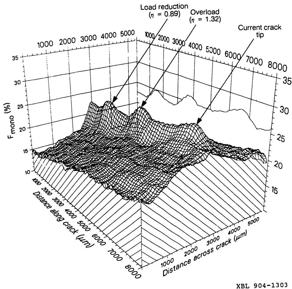
**Fig. 8:** Morphology of the transformation zone, indicated by the volume fraction of the transformed phase,  $F_{\text{mono}}$ , derived from Raman spectroscopy measurements, surrounding a fatigue crack in TS-grade Mg-PSZ ( $K_c \approx 16 \text{ MPa}\sqrt{\text{m}}$ ), following the loading sequence shown in Fig. 7b [10].
