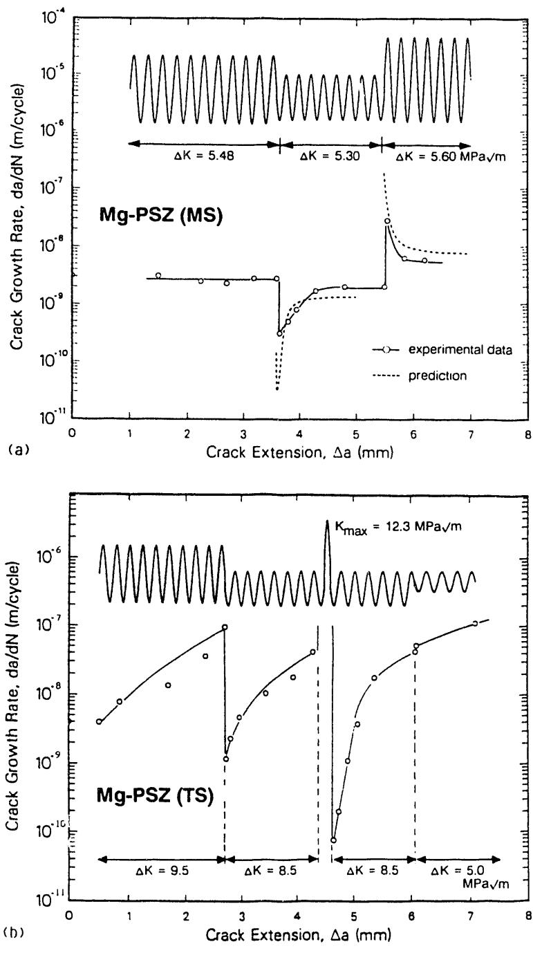
Fig. 7: Transient fatigue-crack growth behavior in a) MS-grade and b) TS-grade Mg-PSZ, showing variation in growth rates following various block loading and tensile overload cycling. Predictions in a) rely on steady-state crack-growth rate data (Fig. 6b) and transformation-zone size measurements (Fig. 8) [10].
