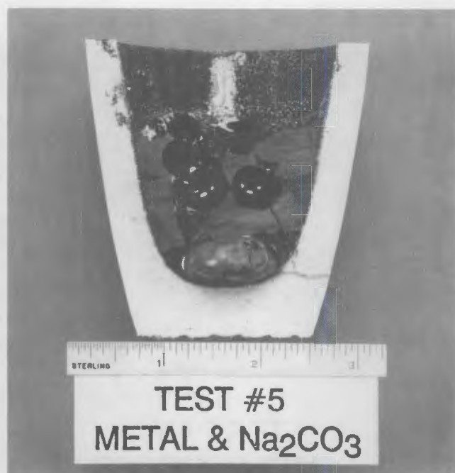
FIGURE 5.5. Cross Section of the Crucible Test 5 Melt
