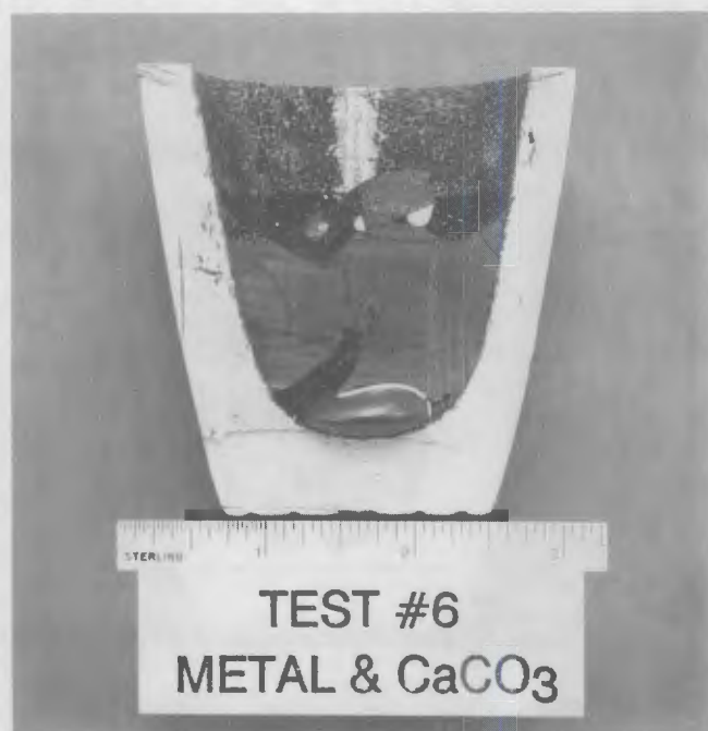
FIGURE 5.6. Cross Section of the Crucible Test 6 Melt
