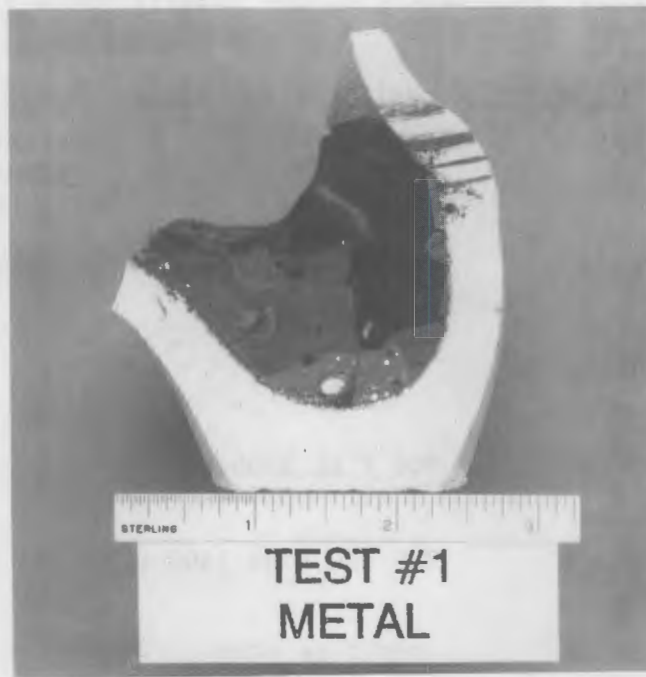
FIGURE 5.1. Cross Section of the Crucible Test 1 Melt
