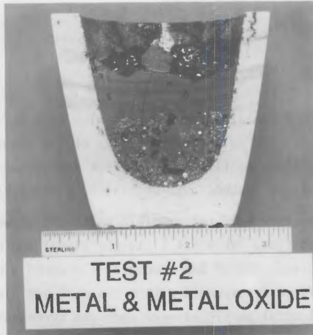
FIGURE 5.2. Cross Section of the Crucible Test 2 Melt
