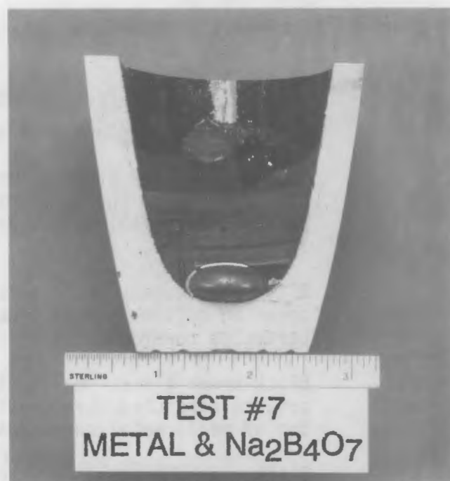
FIGURE 5.7. Cross Section of the Crucible Test 7 Melt
