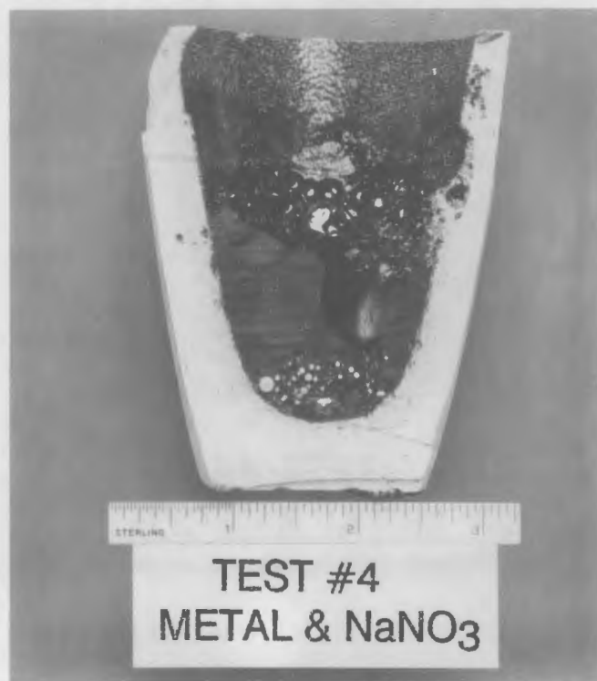
FIGURE 5.4. Cross Section of the Crucible Test 4 Melt
