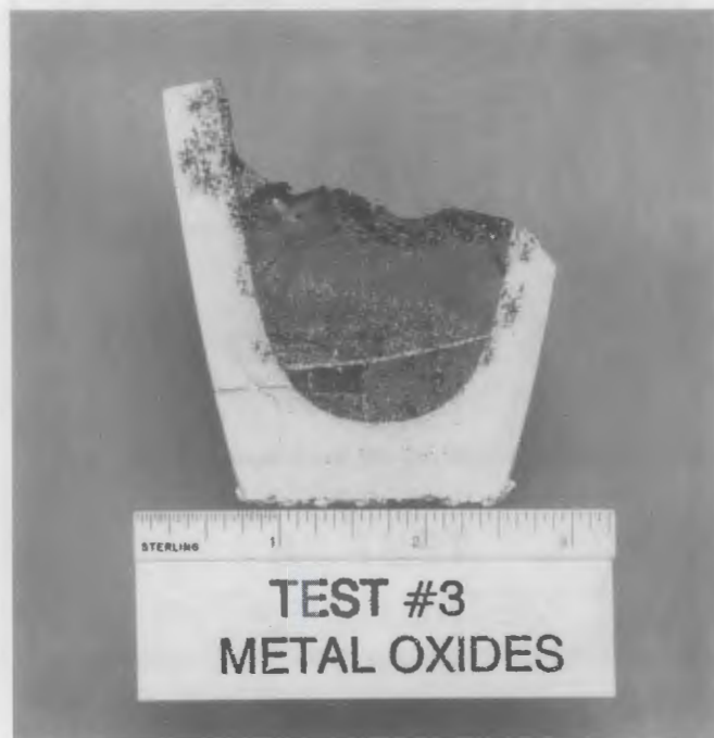
FIGURE 5.3. Cross Section of the Crucible Test 3 Melt
