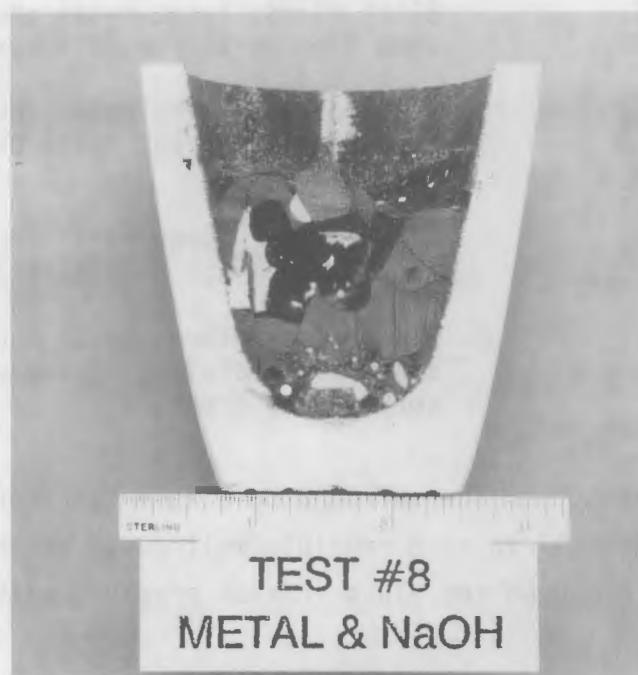
FIGURE 5.8. Cross Section of the Crucible Test 8 Melt
