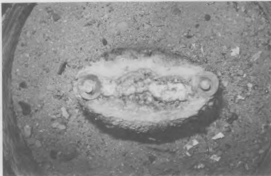
FIGURE 6.7: Direct Metal Short on the Bottom of the BS-INEL-2 Vitrified Block
