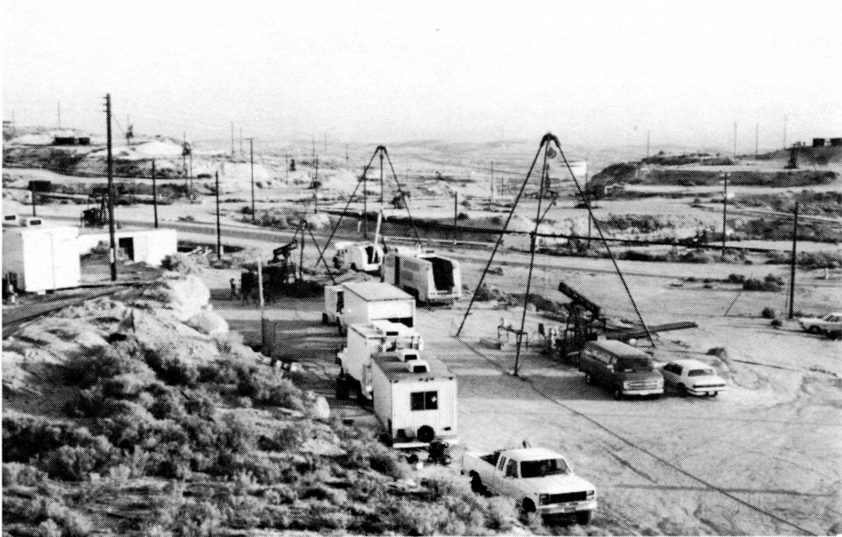
Tripods set up over wells for conducting crosswell seismic studies to image a major fault in the McKittrick field, California – Los Alamos National Laboratory and Chevron Oil Field Research Company
