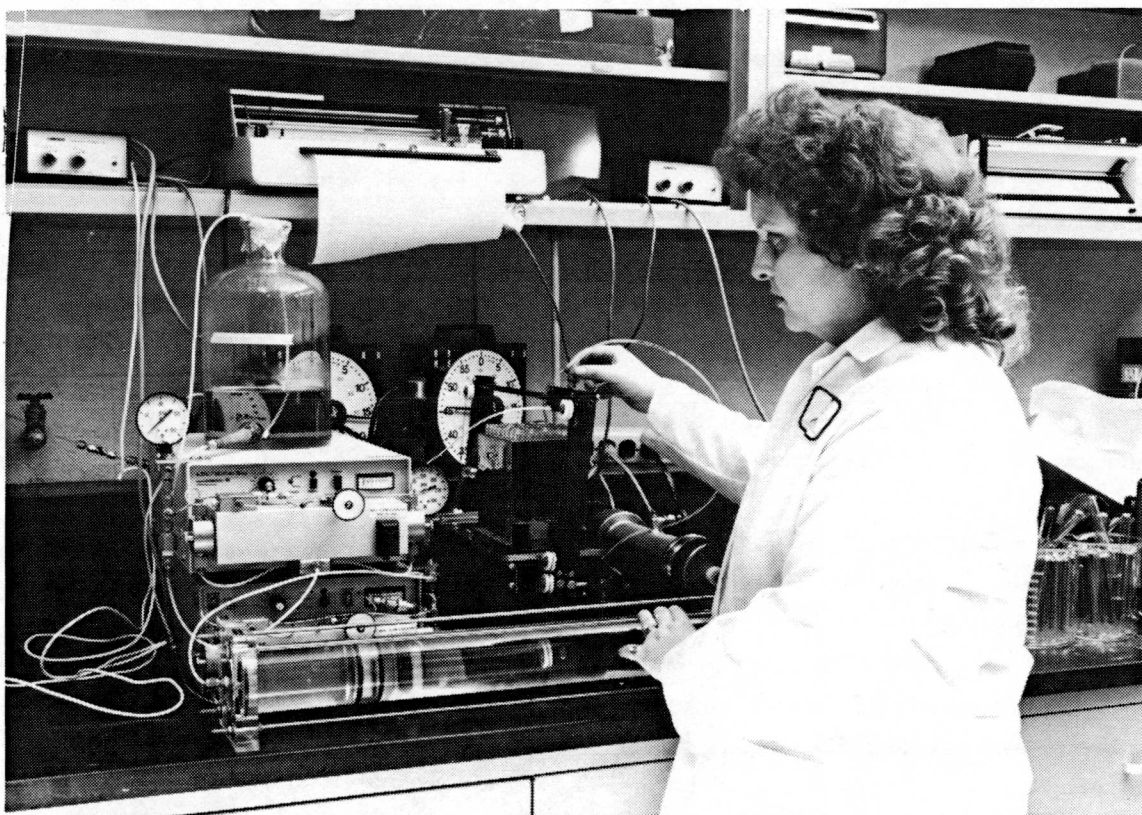
Coreflooding experiment to determine oil recovery by microbial-enhanced waterflooding — National Institute for Petroleum and Energy Research
