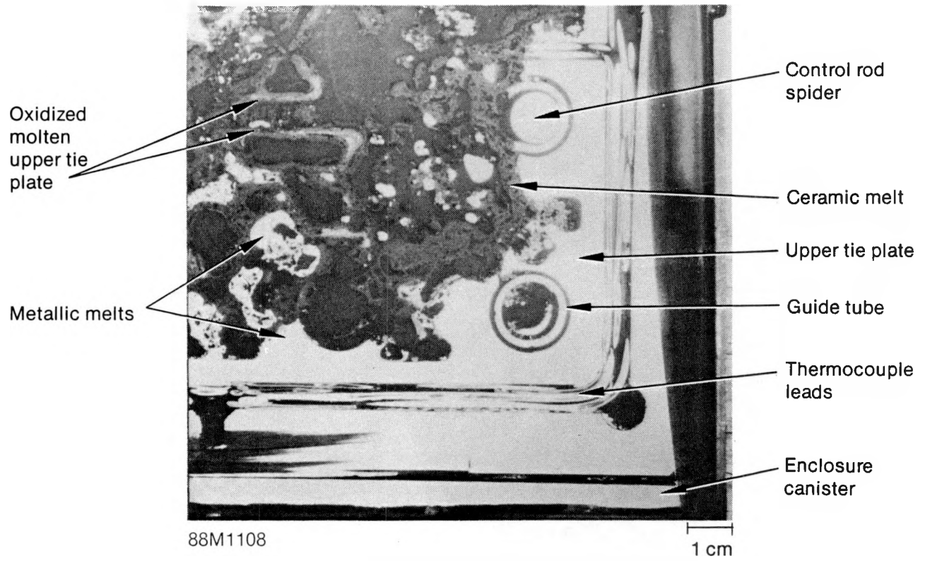
Figure 13. Quarter cross-section through the upper tie plate (1.8 m).
