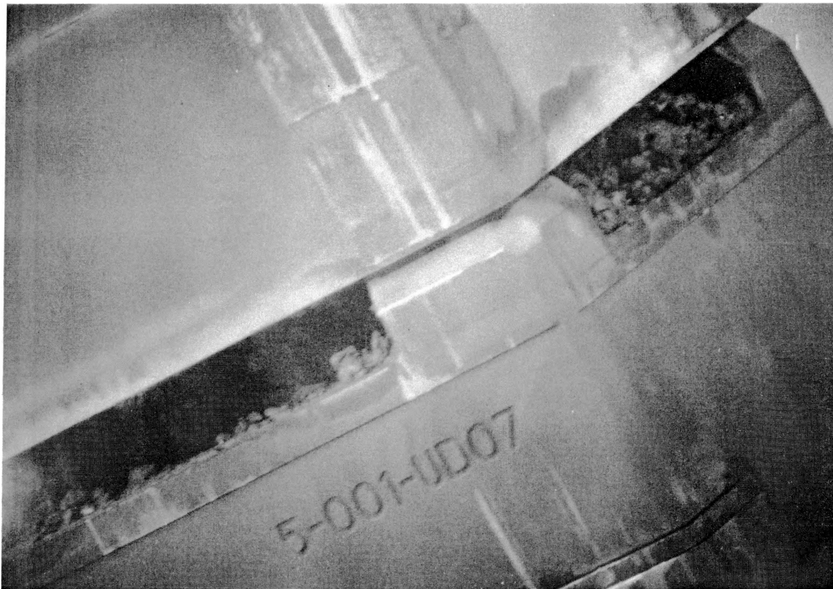
Figure 3. Close-up view of relocated debris in the LP-FP-2 upper end box.
