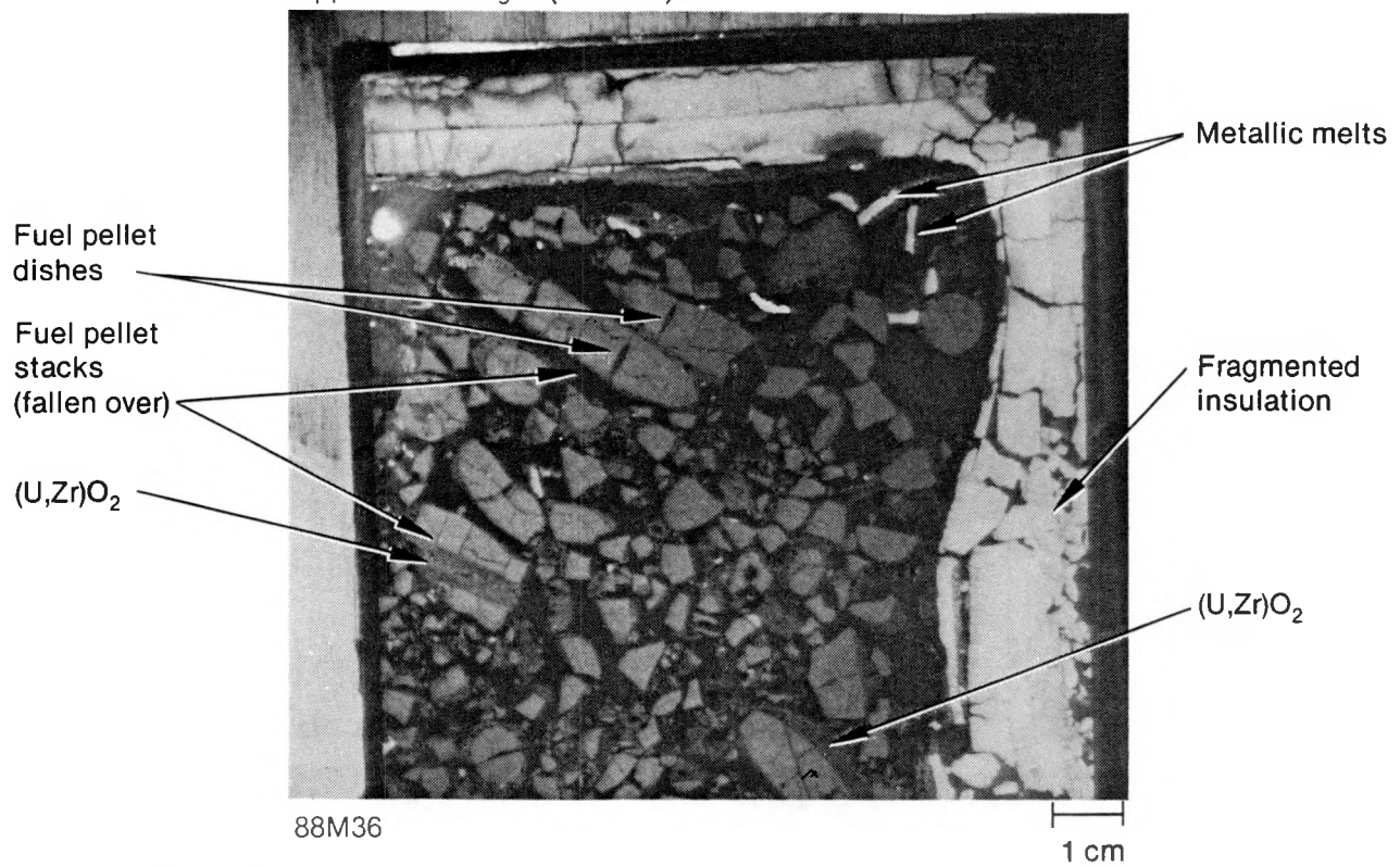
Figure 12. Quarter cross-section through the fuel debris bed (1.2 m).
