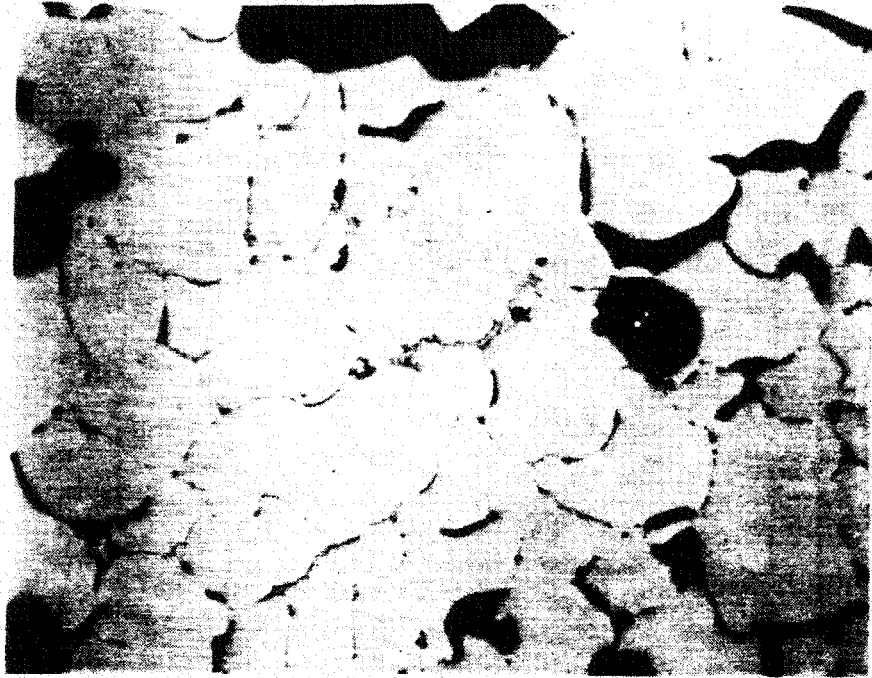
Figure 5. Low porosity region - no grain boundary precipitates
