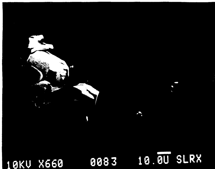
Figure 11. SEM photographs of inclusions in polycrystalline wafer from Semix brick C4-108.
