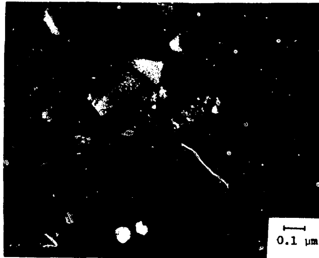
Fig. 4. Helium bubbles in as-implanted and consolidated molybdenum powder compact (TEM).
