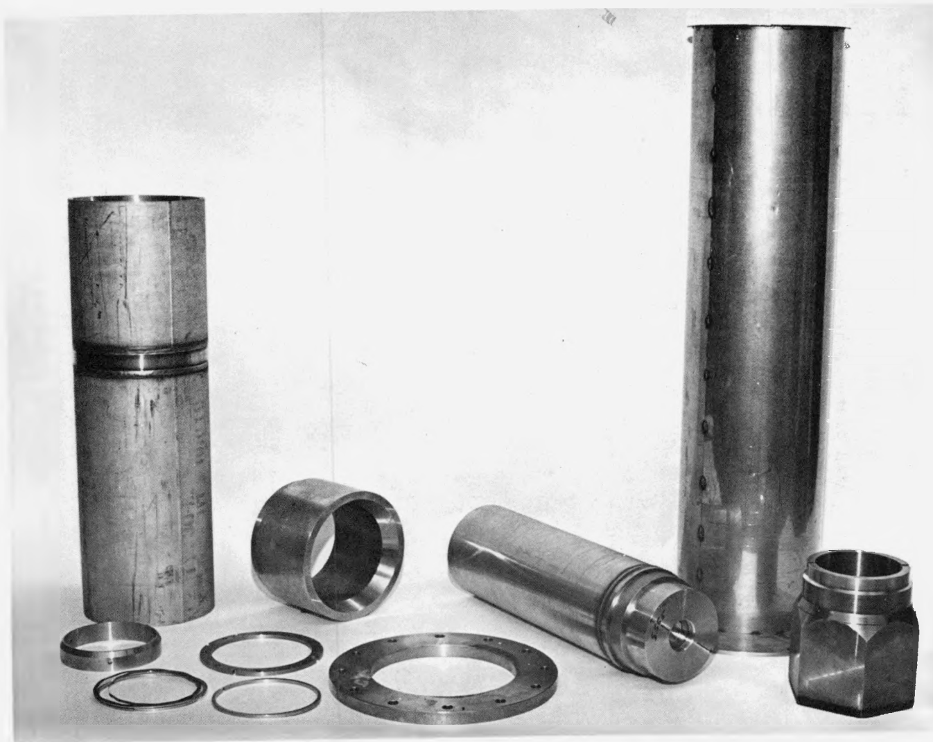
Fig. 3-7. Test facility parts for fuel element ring seal test
