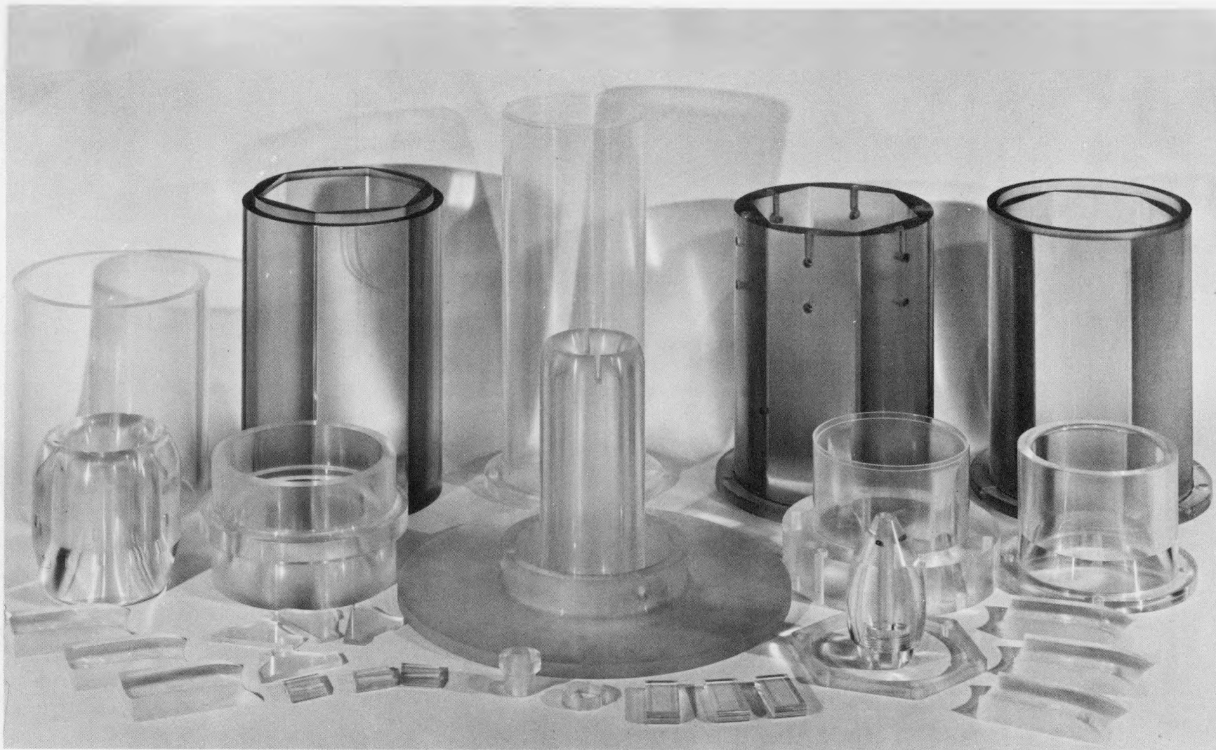
Fig. 2-7. Fuel element nozzle flow test parts
