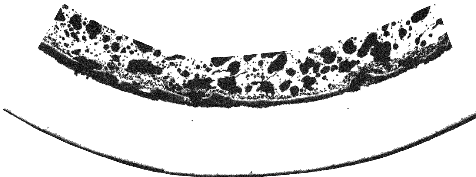
Fig. 9. Lack of Cladding Penetration in This Region of the 88-04 Specimen May Be Attributed to the Presence of the Thick Layer(s) on the Fuel Outer Surface. (77X, AP, MCT 244039)
