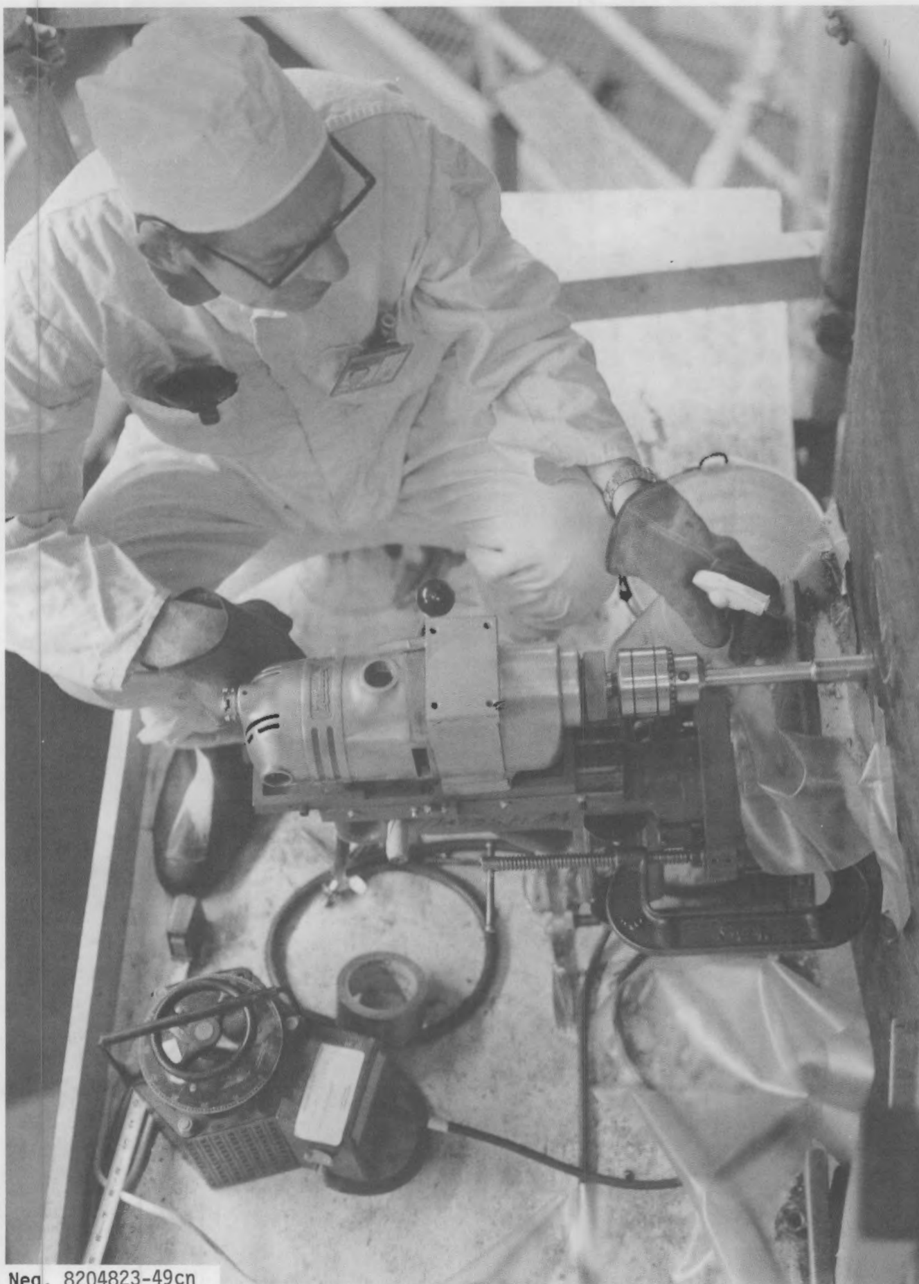
FIGURE 6D. Drilling Core Sample from Channel Head
