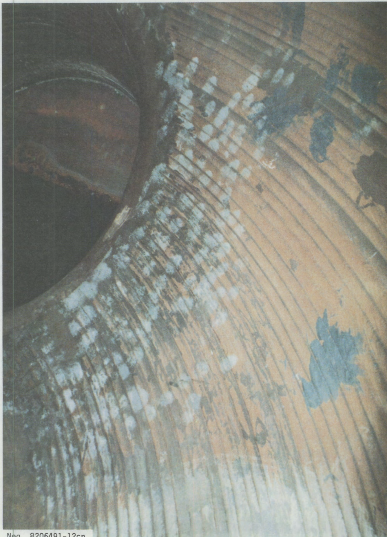
FIGURE 72. Splotchy Appearance of Film
