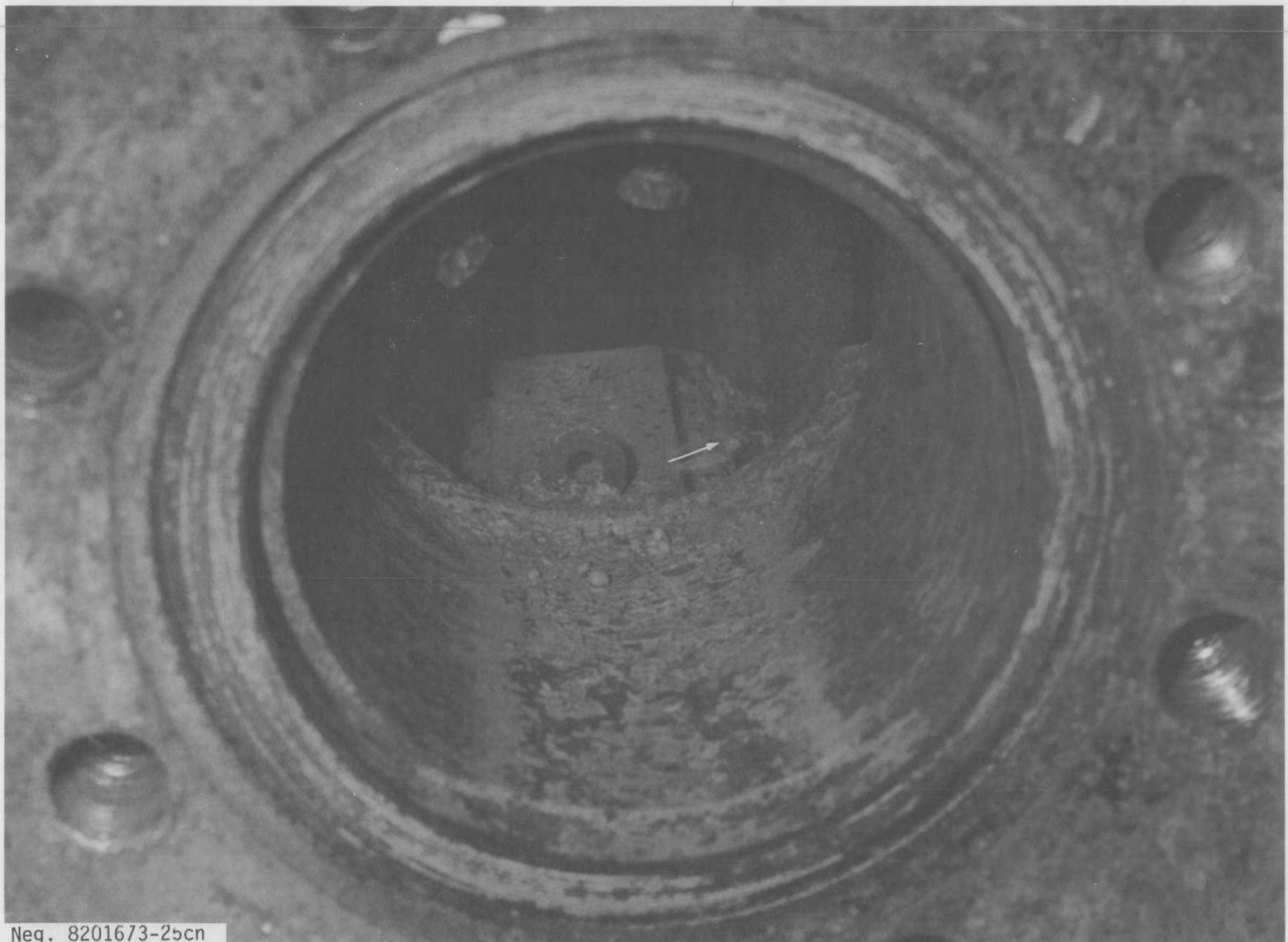
FIGURE 46. Separated Support Plate Piece at Lower Handhole
