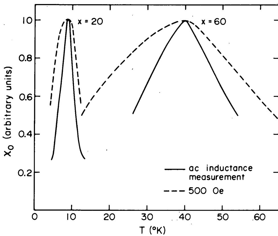
Fig. 4. Susceptibility (in arbitrary unit) as a function of temperature measured in "zero" field and in 500 Oe for  $x = 20$  and 60 samples.
