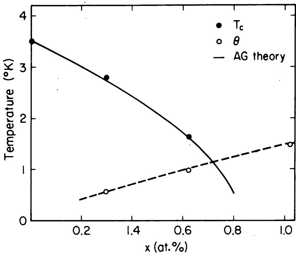
Fig. 2. The dependence of  $T_c$  and  $\theta$  on Gd concentration in  $\text{La}_{80}\text{Au}_{20}$  matrix.
