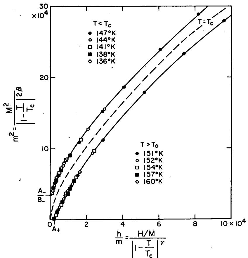
Fig. 1. The normalized magnetization  $m^2$  versus normalized inverse susceptibility  $\chi_o^{-1}$  for temperatures around  $T_c$ . The dashed line indicates asymptotic behavior of the two curves for large  $m$  above and below  $T_c$ .
