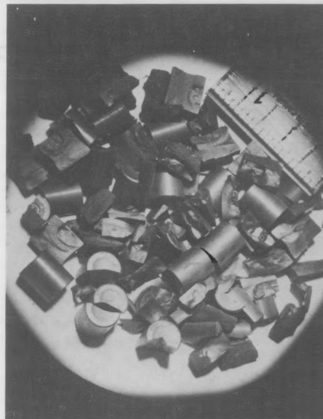
FIGURE 41. Fuel Fragments from Rod Section 3B5A Before Sieve Shaking
