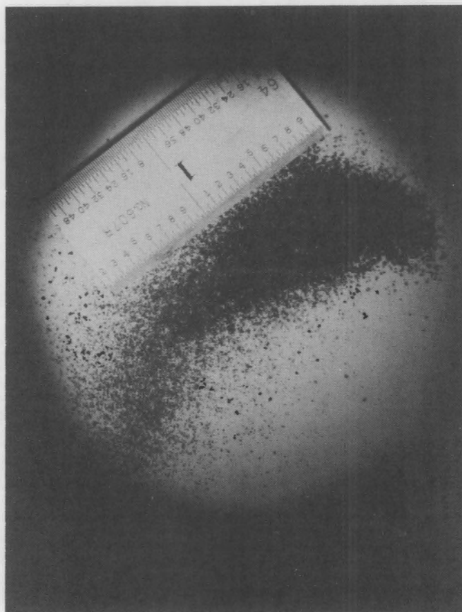
FIGURE 48. Rod Section 3B5A Fuel Fragments from Receiver ( <0.0117 in., <300\text{ }\mu\text{m} )
