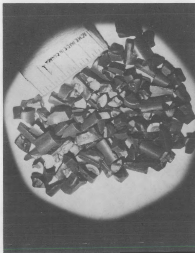
FIGURE 43. Rod Section 3B5A Fuel Fragments from Screen 2 (0.157 in., 4.0 mm)
