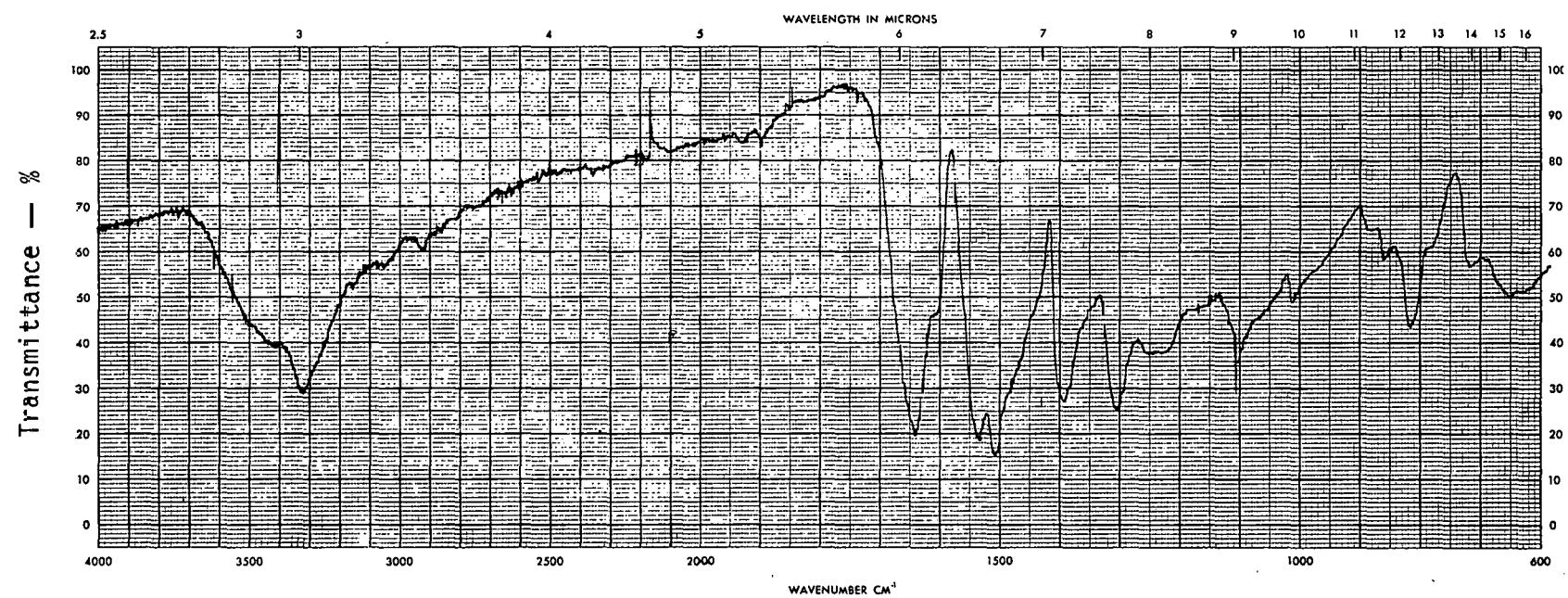
Fig. 1. Infrared spectrum of Kevlar 49 yarn.
