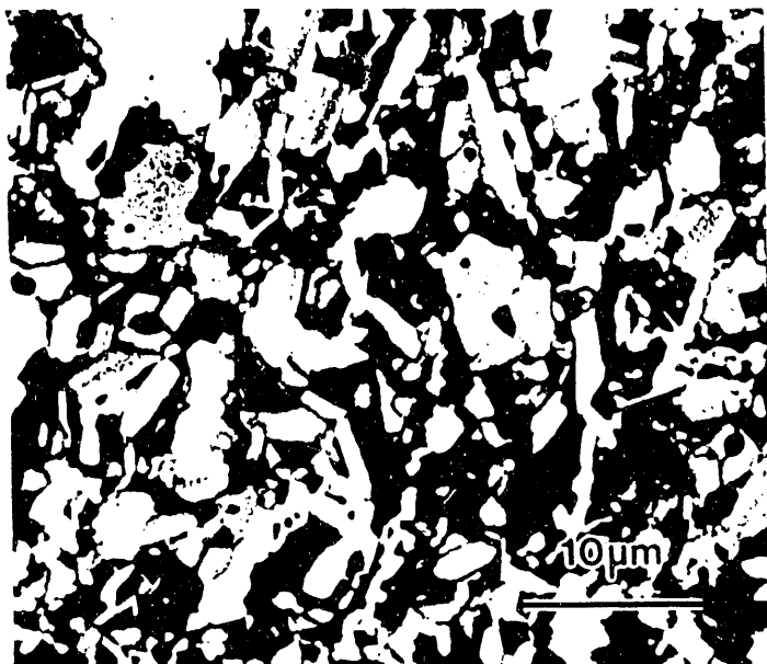
Fig. 1 SEM backscattered electron micrograph of the Tl(1223) tape annealed in the solid state at 850°C for 36 hours.
