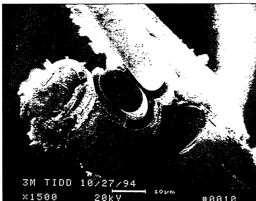
Figure 18e — Additional Micrographs Illustrating The Morphology Of The Confinement Fibers In The 3M CVI-SiC Composite Filter Matrix After 1705 Hours Of Exposure To The PFBC Gas Environment
