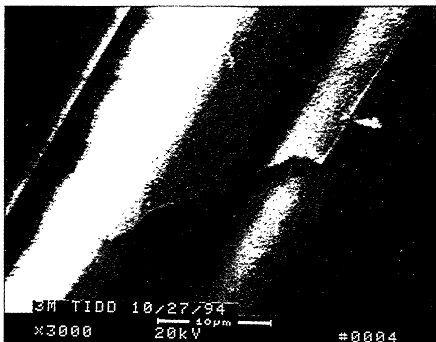
Figure 14b – Higher Magnification Micrographs Of The Confinement Layer Fibers
