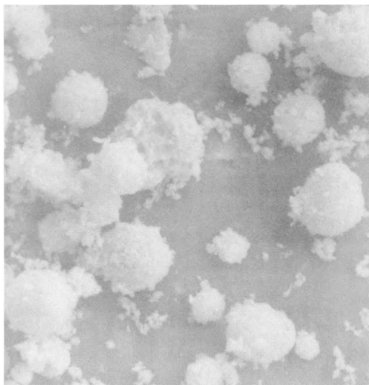
FIGURE 5.11 Scanning Electron Microscope Photograph of Recycled Powder Produced at 150°F (600X magnification)
