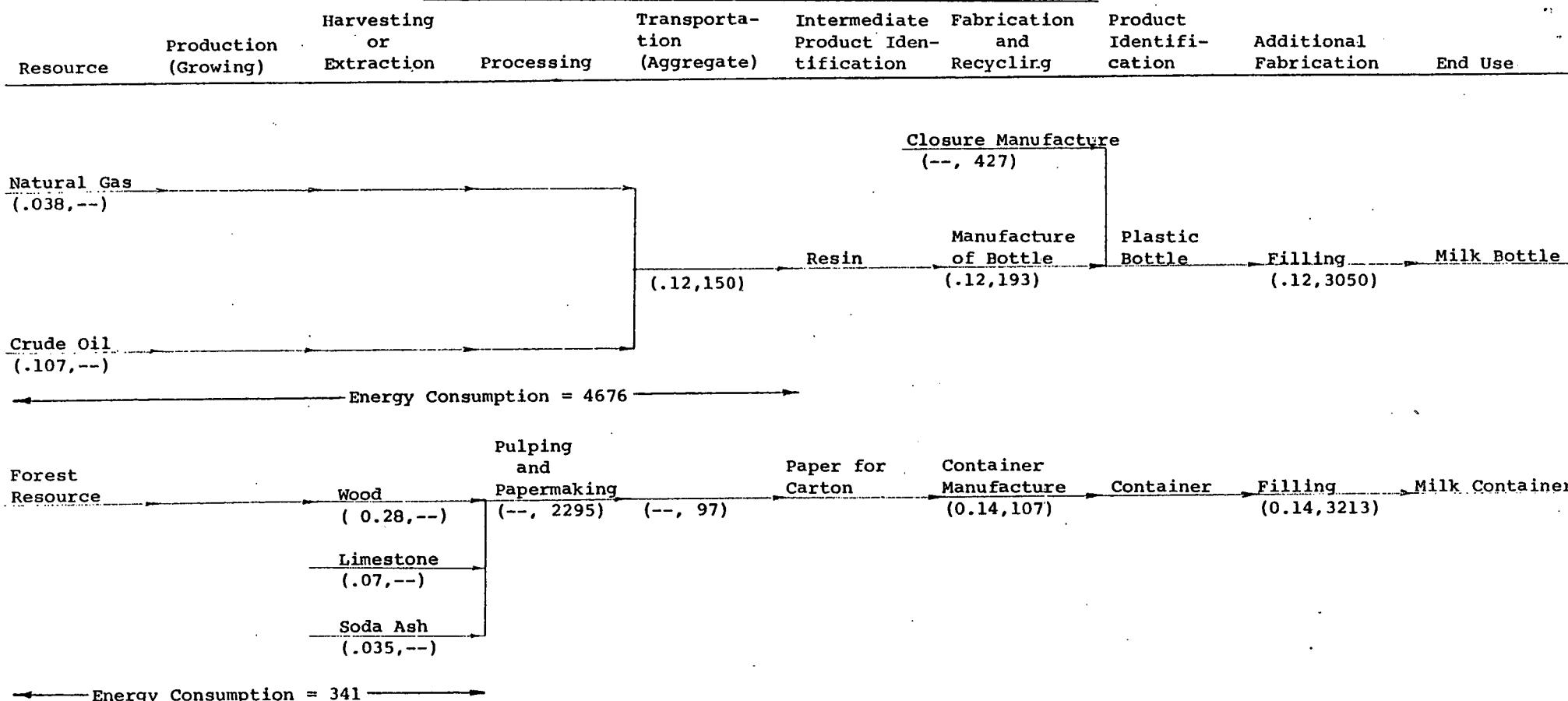
NOTE: Numbers in the parentheses below the activity links refer to mass flow in lb and energy requirement in Btu respectively for the corresponding steps in the manufacture of one half gallon milk containers.
