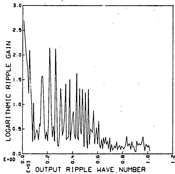
Figure 2. Maximum ripple gain spectrum for the CYCLOPS laser system through the third B-module for  $11.5 \text{ GW/cm}^2$  output intensity.
