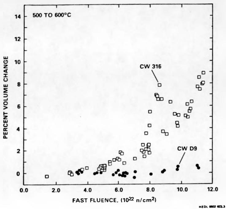
FIGURE 1. Swelling of Cold Worked D9 and 316 SS Cladding Versus Fast Fluence. Data are immersion density measurements made on irradiated fuel pin cladding from which the fuel had been removed.
