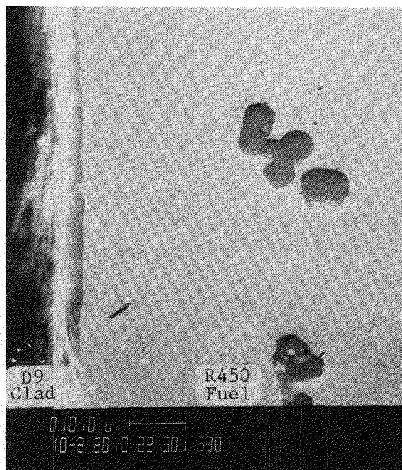
Fig. 11. Interfaces between U-15Pu-11Zr (R450) Archive Fuel and Clads after 300 h at 757°C (Test DC4).
