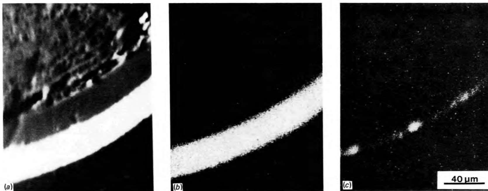
Fig. 23. X-ray displays of fissile particle, ZrC-buffered \text{UO}_2 kernel Triso coated, in Fig. 22 which was irradiated in HRB-15a fuel rod 2. (a) Backscattered electron image of iPyC-SiC interface. (b) Si K\alpha . (c) Pd L\alpha .
