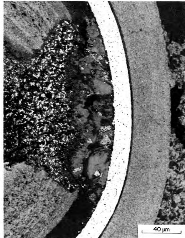
Fig. 3. High magnification of ZrC coating from Fig. 1(a) showing (a) cold side of the particle and (b) hot side. The "peppery" appearance of ZrC is thought to be a chemically induced porosity due to residual chlorine for the coating run.
