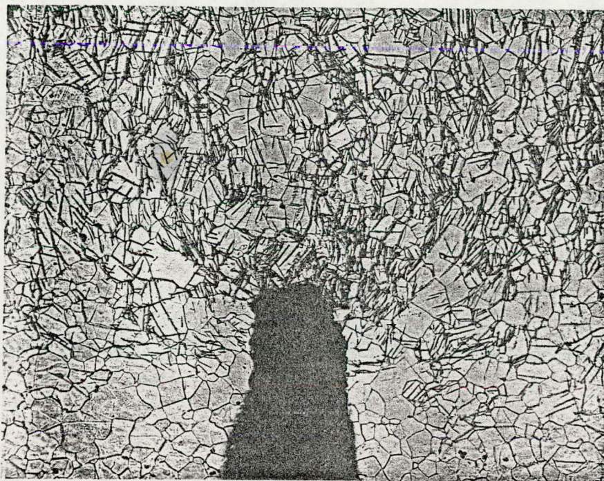
Fig. 5. Stress-induced hydride at the root of a notch in 845 ppm H_2 alloy, loaded to K_I = 8.4 \text{ MN}\cdot\text{m}^{-3/2} for 260 hours at room temperature.
