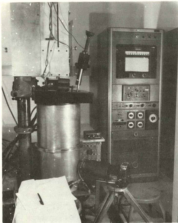
Fig. 4-36. Hoffman furnace set-up showing furnace control panel, optical pyrometer, 35mm camera, tripod, and intervalometer
