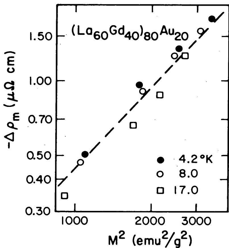
Fig. 4. Negative magnetoresistivity of the 40 at. % sample vs its magnetization squared. Dashed line is an arbitrary line of slope unity.
