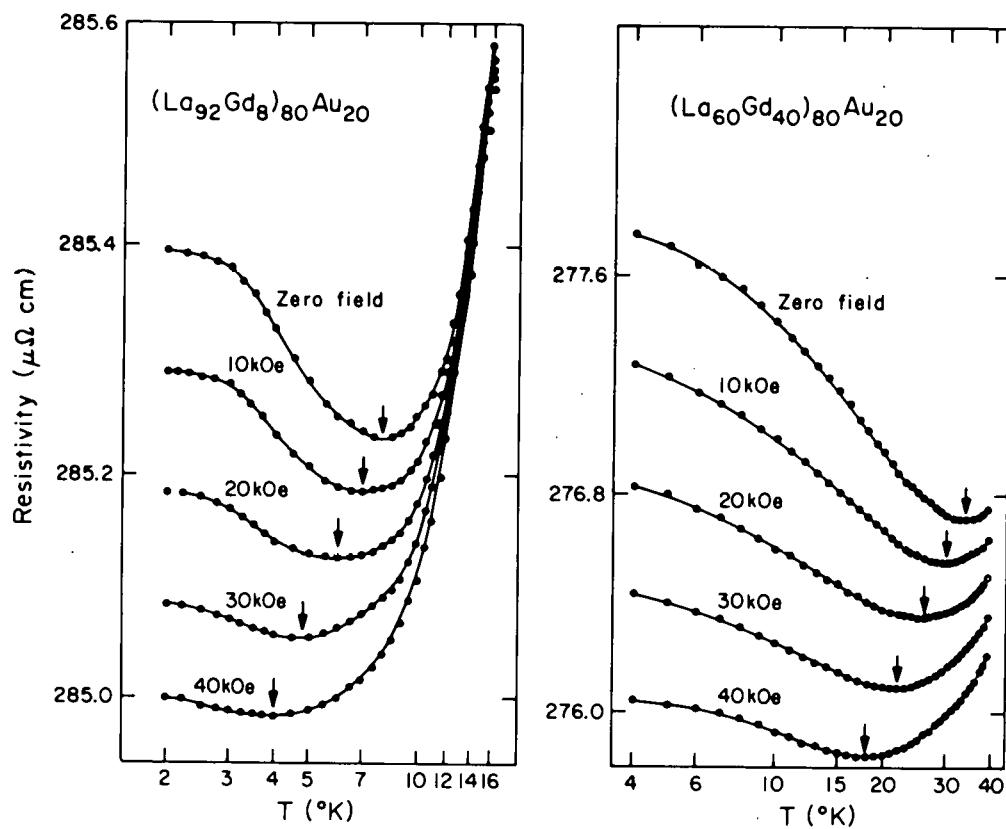
Fig. 1. Resistivity of  $x = 8$  and 40 samples as a function of temperature and magnetic field. Arrows indicate positions of resistivity minima.
