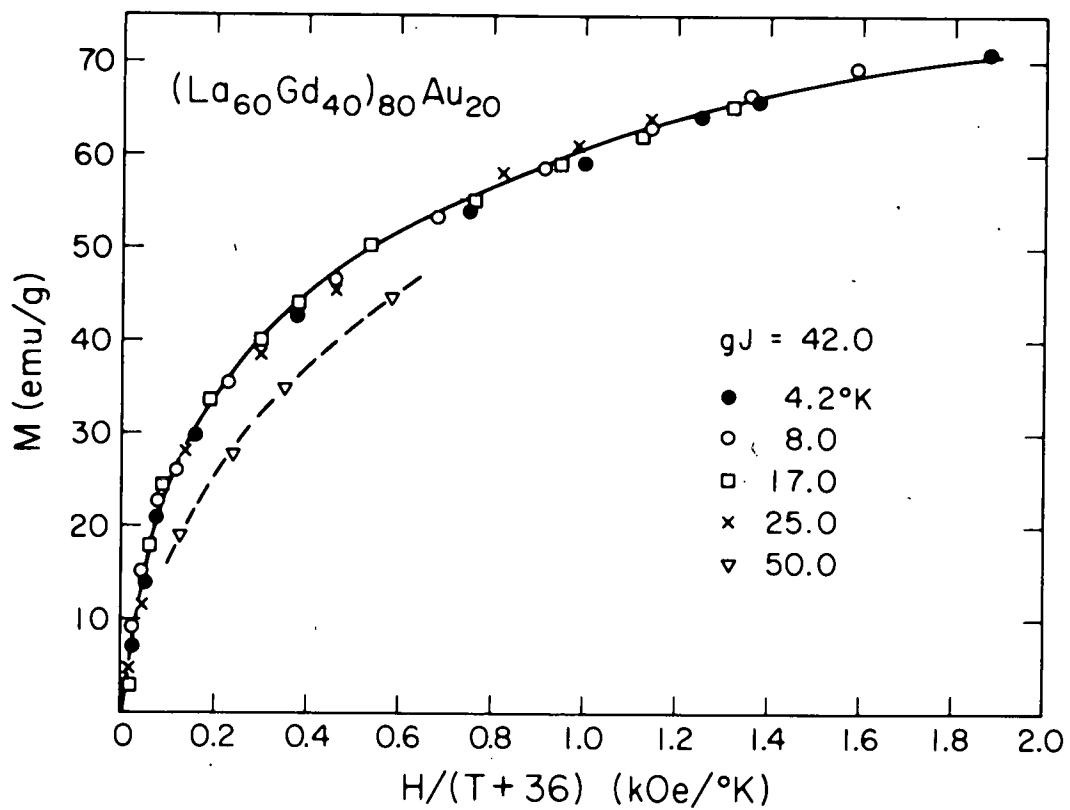
Fig. 3. Magnetization of the 40 at.% sample vs  $H/(T + 36)$ . Solid line is the Brillouin function fit with  $g = 2$ ,  $J = 21$ , and  $\theta_c = 36^\circ\text{K}$ . Dashed line shows deviation from such relation.
