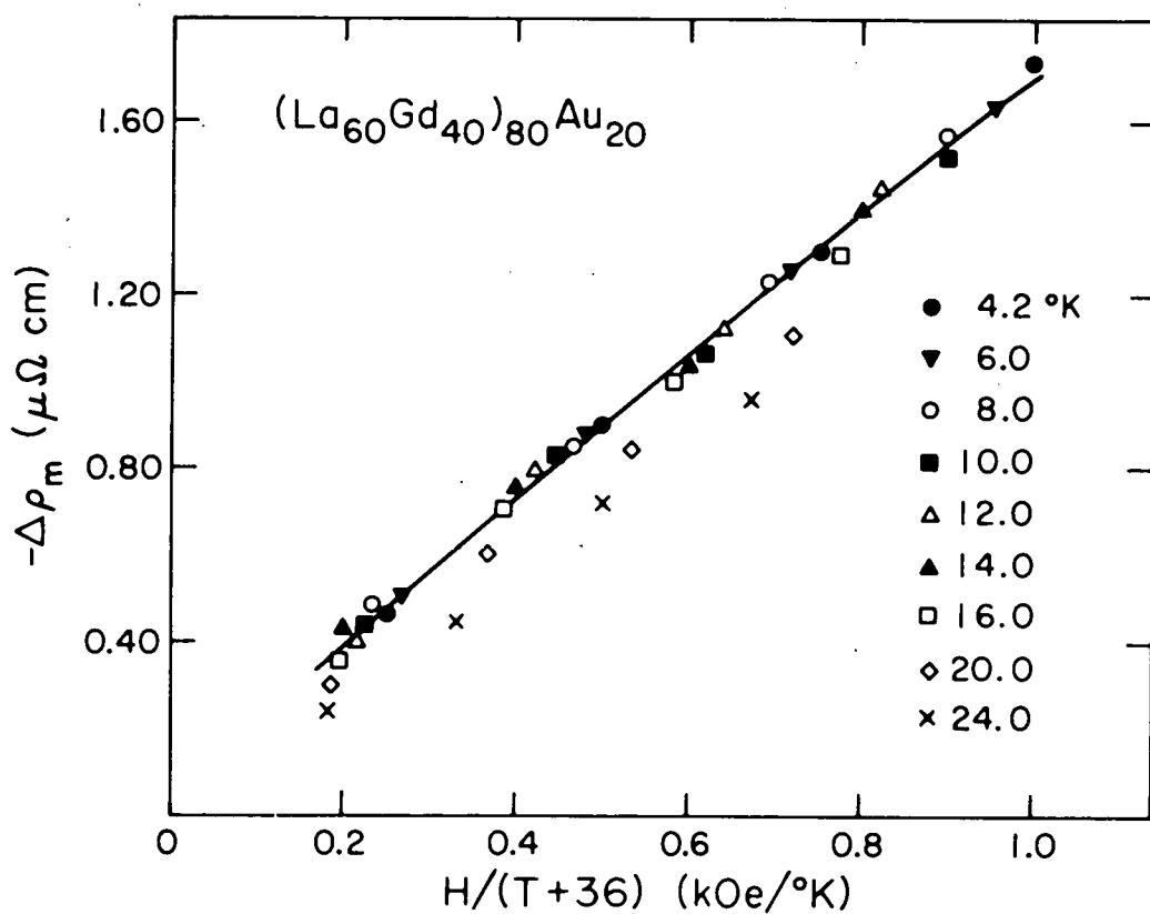
Fig. 2. Negative magnetoresistivity of the 40 at.% sample vs  $H/(T + 36)$ . Solid line indicates the general behavior below 16 $^{\circ}$ K.
