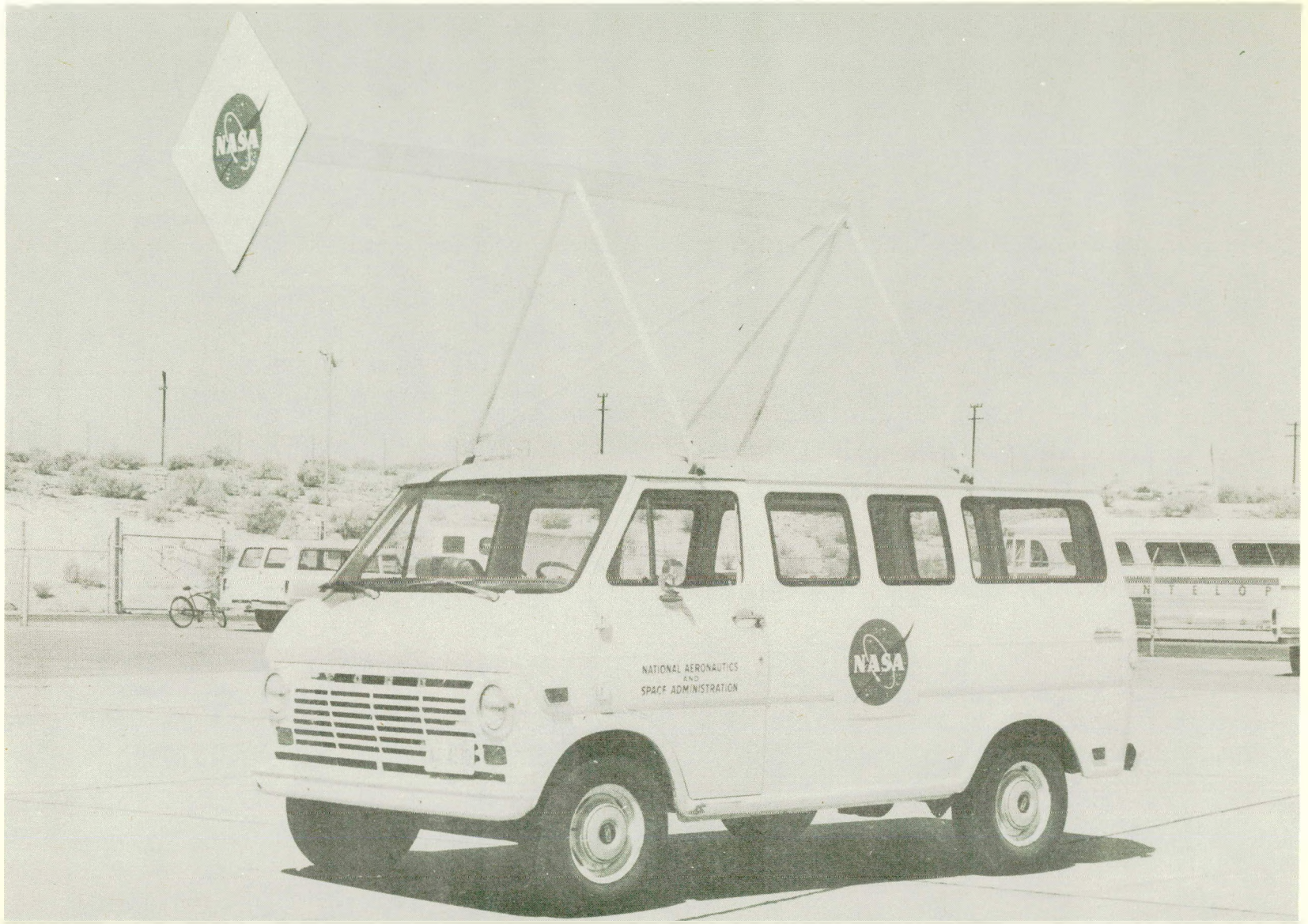
Figure 3. Carrier vehicle with flat plate and supporting structure.
