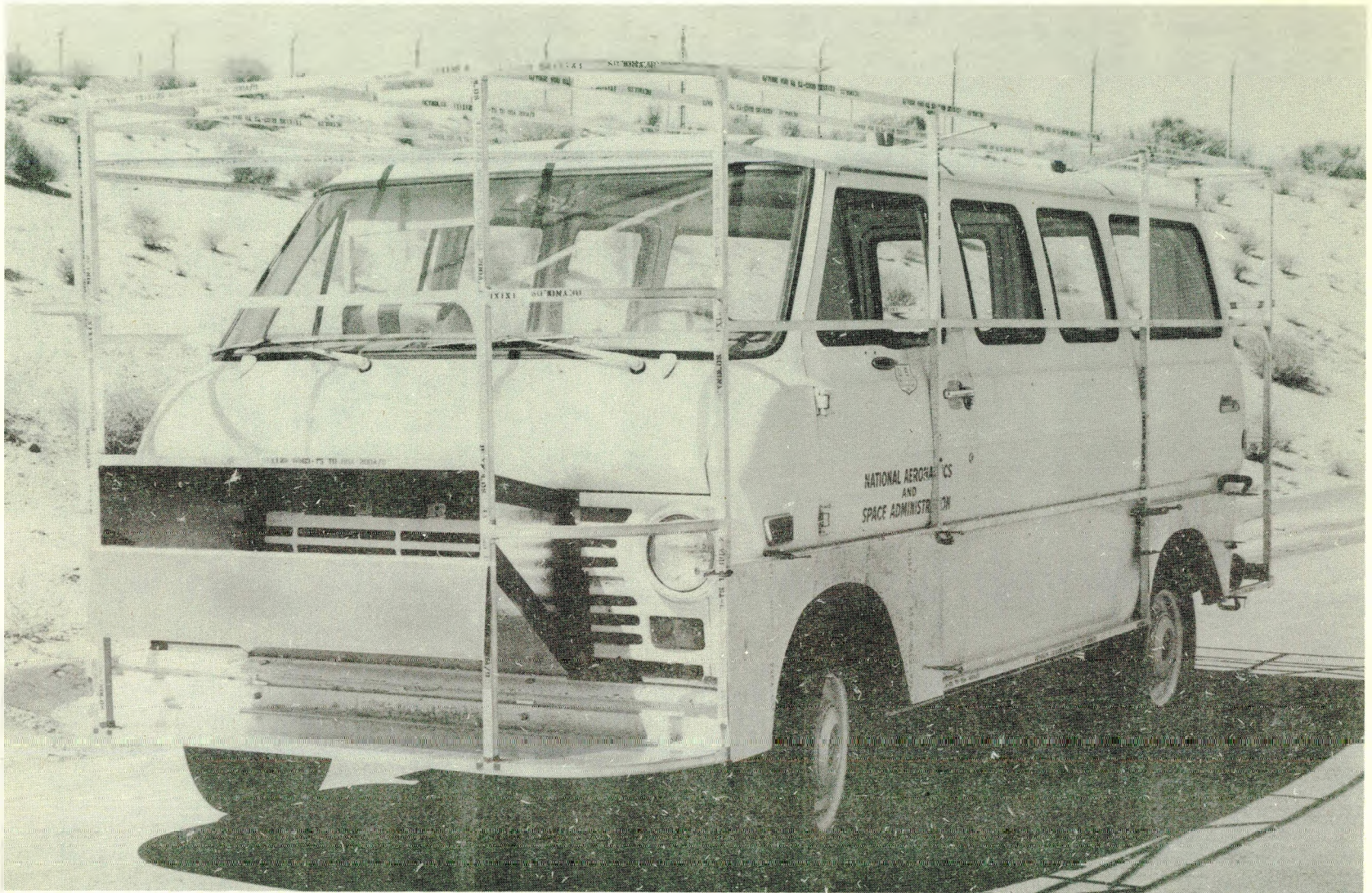
Figure 5. Carrier vehicle with aluminum subframe.
