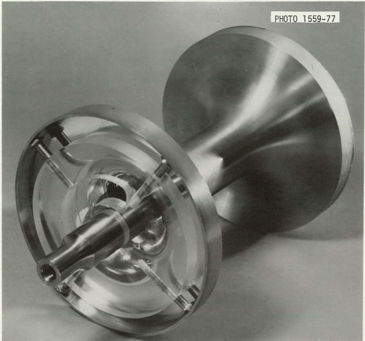
FIG. 1. Mounted concentric cylinder electrodes.
