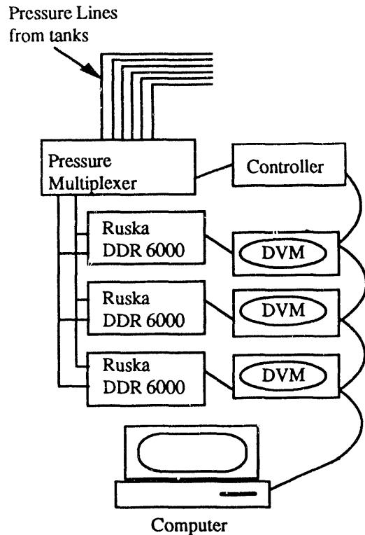
With all sensors reading the same pressure, comparisons can be made with each reading. Since the system averages the readings over time and calculates the standard deviations, the standard deviation is used to measure stability. Therefore, an individual instrument's measurement must meet two criteria:
