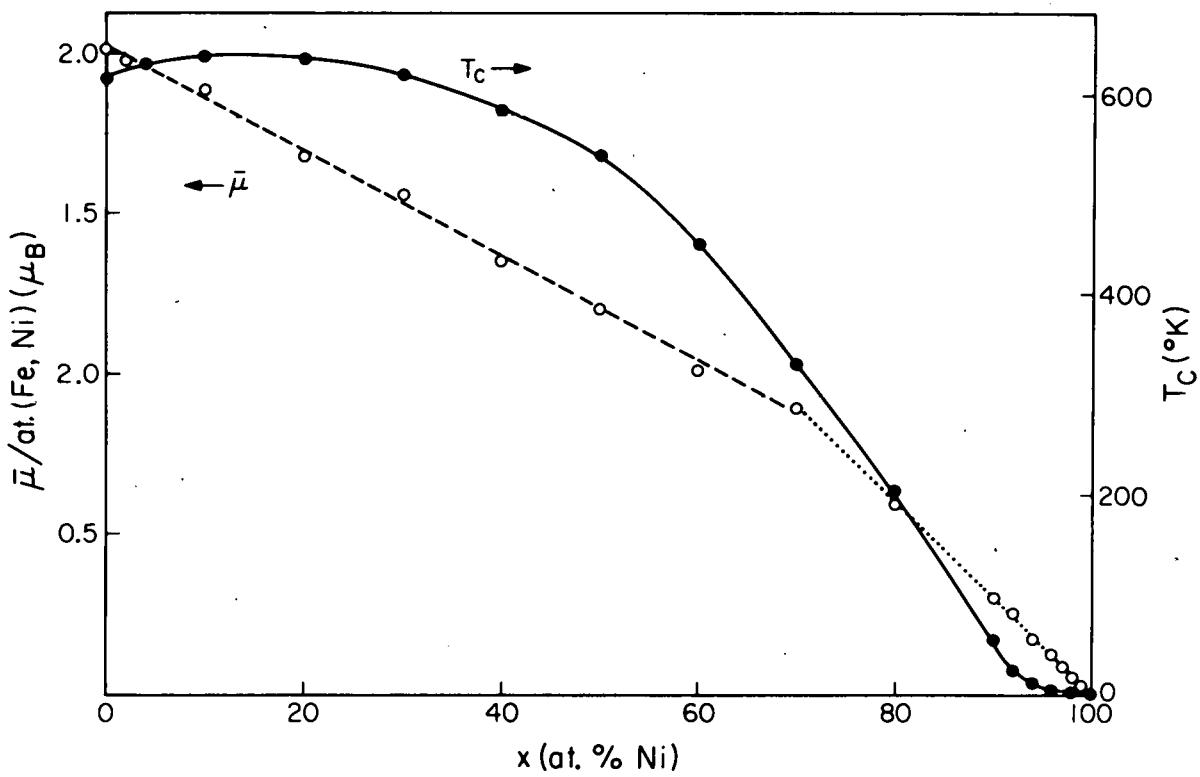
Fig. 1. Variation of the Curie temperature  $T_c$  and of the mean magnetic moment per transition metal atom  $\bar{\mu}/\text{at. (Fe, Ni)}$  as a function of the Ni content  $x$  in amorphous  $(\text{Fe}_{100-x}\text{Ni}_x)_{79}\text{P}_{13}\text{B}_8$  alloys.
