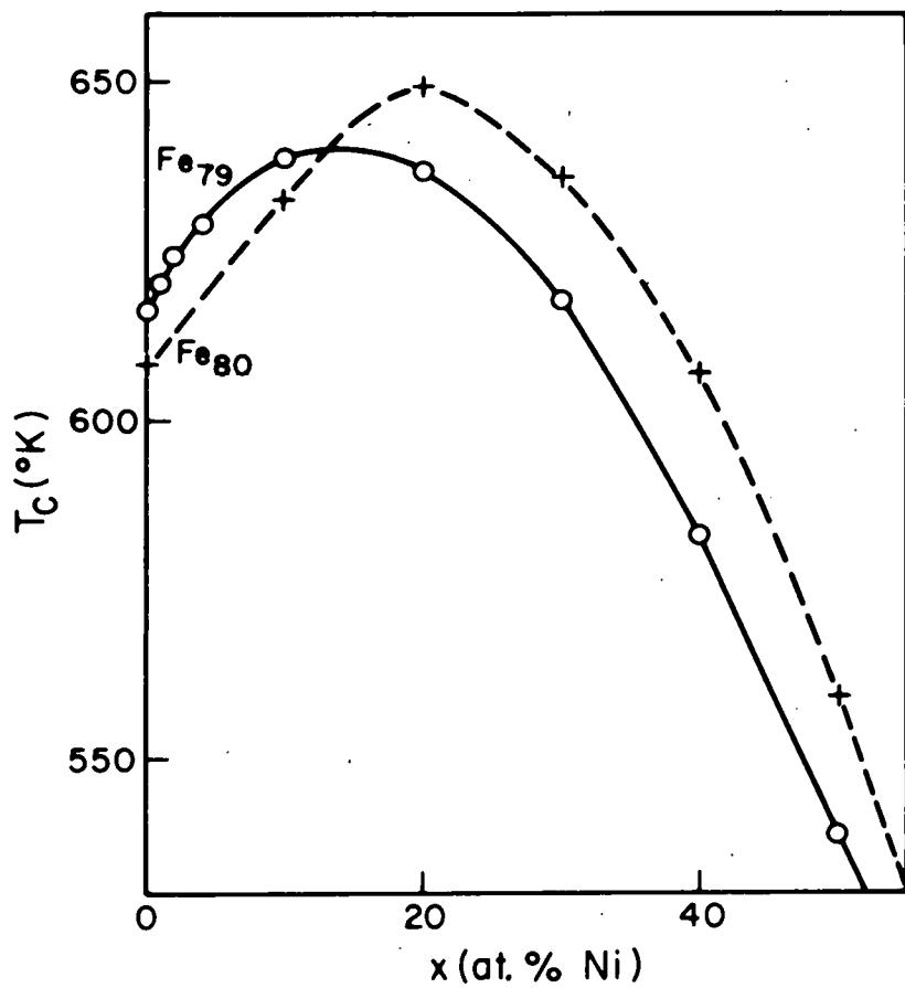
Fig. 5. Curie temperature as a function of Ni content in amorphous  $(Fe_{100-x}Ni_x)_{79}P_{13}B_8$  (0) and  $(Fe_{100-x}Ni_x)_{80}P_{12}B_8$  (+) alloys.
