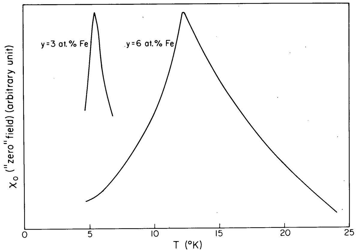
Fig. 3. Magnetic susceptibility (in arbitrary unit) as a function of temperature in "zero" field for  $y = 3$  and 6 at. % Fe in amorphous  $(\text{Ni}_{100-y}\text{Fe}_y)_{79}\text{P}_{13}\text{B}_8$  alloys.
