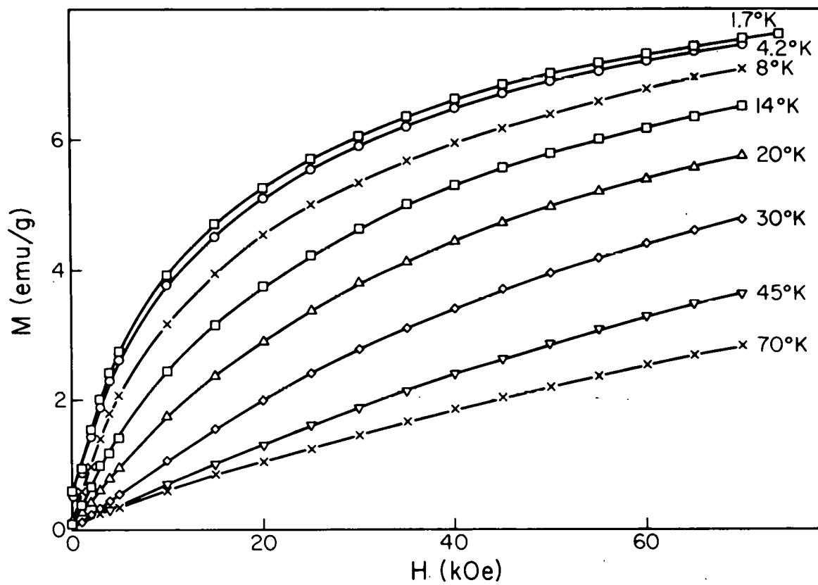
Fig. 2. Magnetization versus applied field at low temperature in amorphous  $(\text{Ni}_{98}\text{Fe}_2)_{79}\text{P}_{13}\text{B}_8$  alloy.
