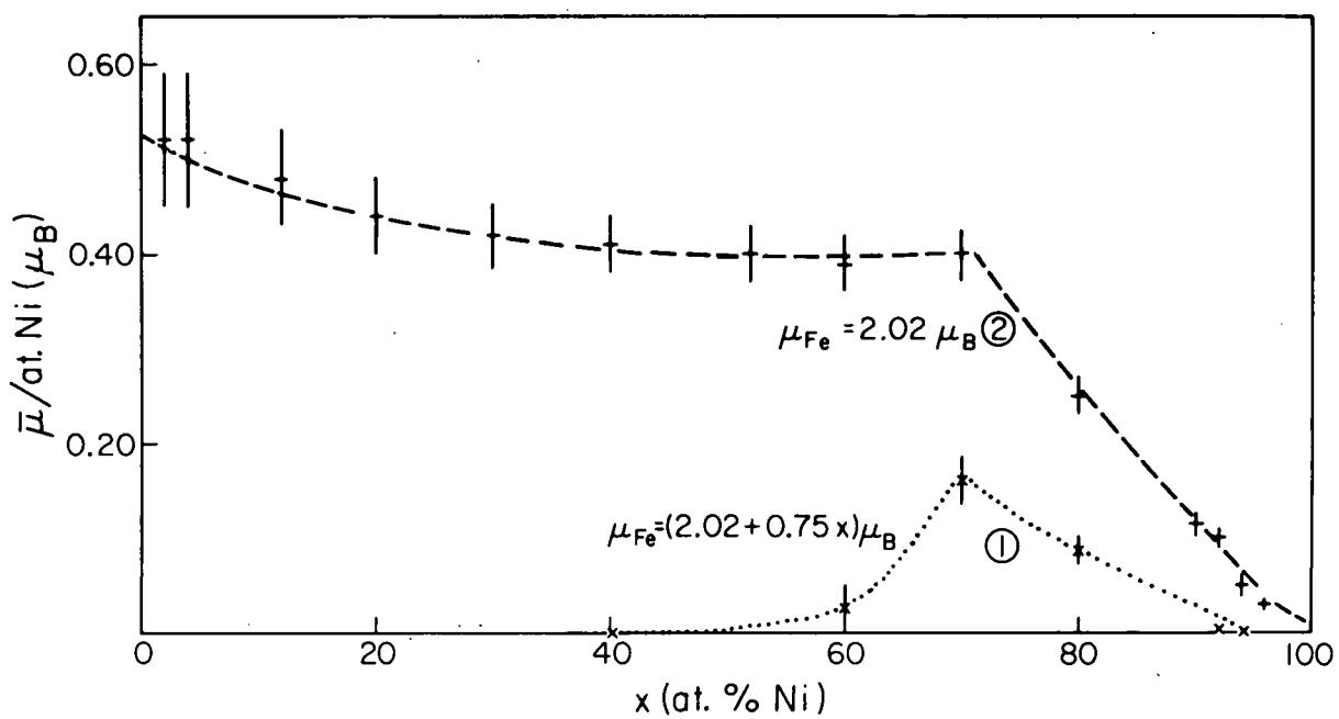
Fig. 6. Estimate of the magnetic moment per Ni atom as a function of Ni content in amorphous (Fe<sub>100-x</sub>Ni<sub>x</sub>)<sub>79</sub>P<sub>13</sub>B<sub>8</sub> alloys.
