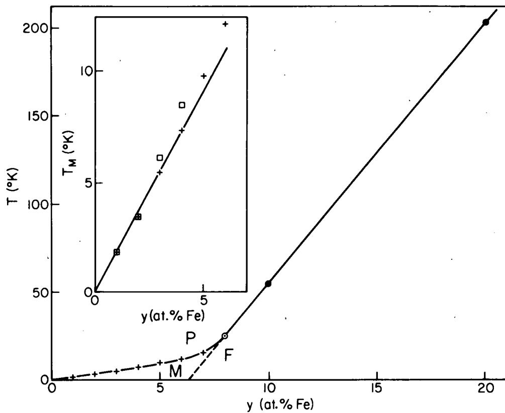
Fig. 4. Ordering temperatures (see text) as a function of Fe concentration in amorphous  $(\text{Ni}_{100-y}\text{Fe}_y)_{79}\text{P}_{13}\text{B}_8$  alloys.
