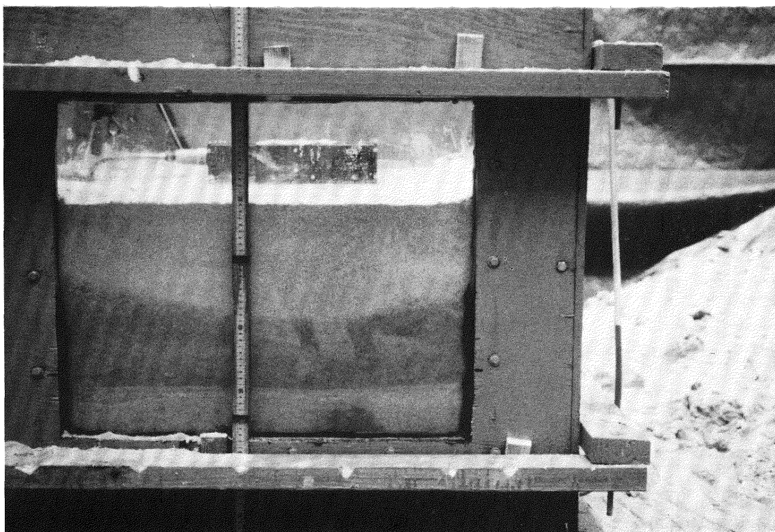
Figure 6.11. Technos Sandbox Showing 900 MHz Antenna.
