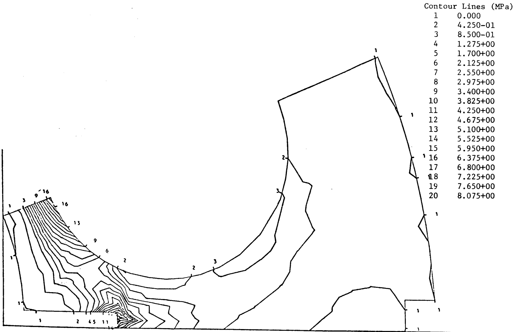
Figure 5 Maximum principal in-plane residual stress for 8-hole element.
