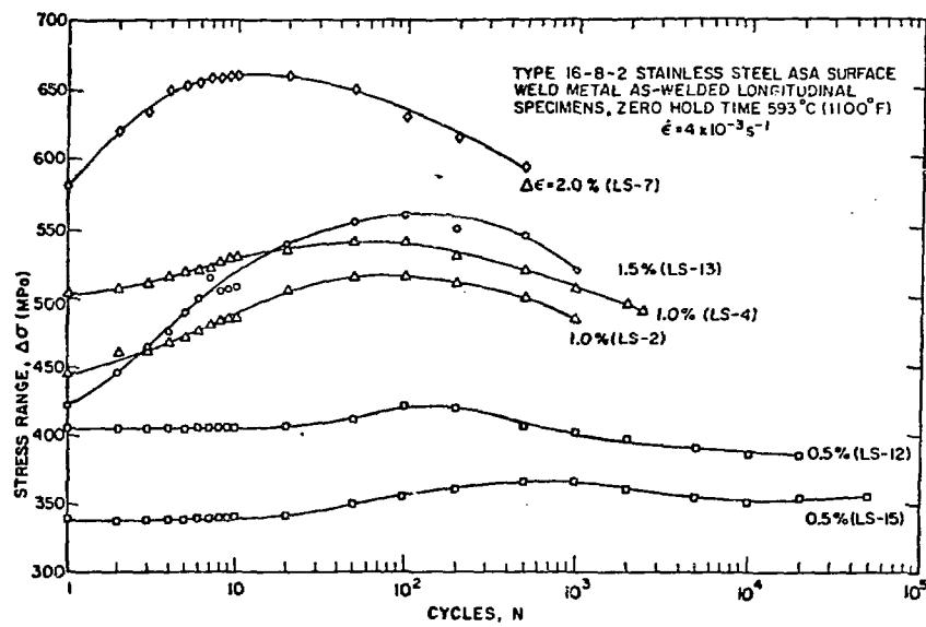
Fig. 6 -- Changes in Stress Range during Reversed Strain Cycling for Surface Weld Metal (Specimen Numbers in Parentheses). MSD-63951.
