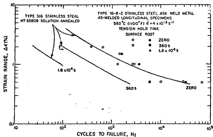
Fig. 5 — Total Strain Range vs Cycles to Failure for Type 16-8-2 Stainless Steel ASA Weld Metal Compared with Type 316 Stainless Steel Baseline Data, MSD-63949.
