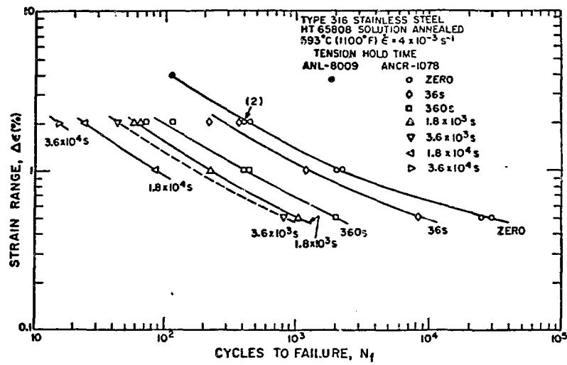
Fig. 1 -- Total Strain Range vs Cycles to Failure Showing Effect of Tension Hold Time on Fatigue Life for Type 316 Stainless Steel Base-line Data (Open Symbols from Ref 12, Solid Symbol from Ref 13. MSD-63754.
