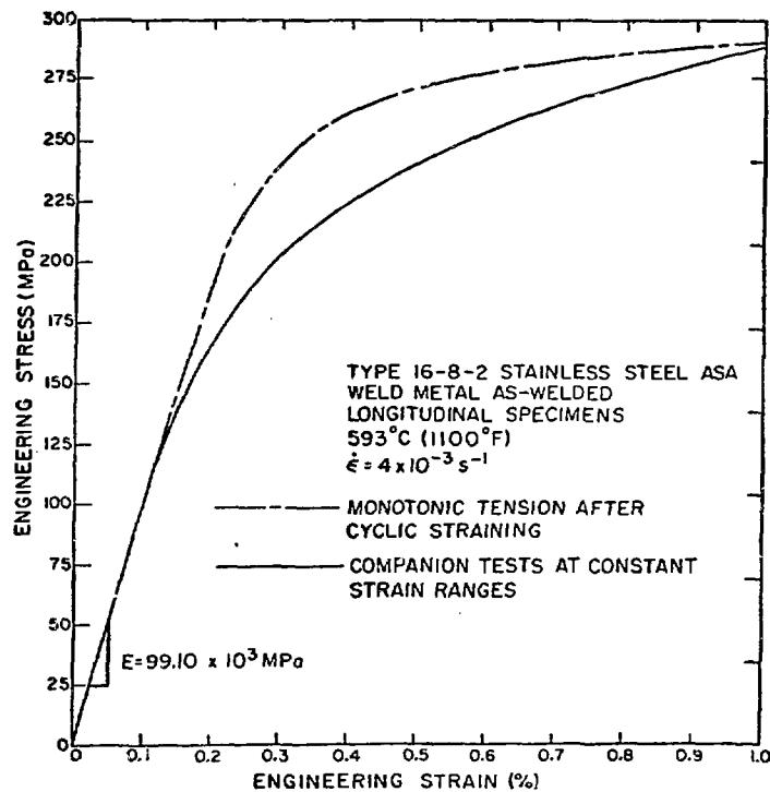
Fig. 8 -- Cyclic Stress-Strain Curves from Constant-amplitude Continuous-cycling Fatigue Tests and Monotonic Tension Test after Cyclic Straining. MSD-63952.
