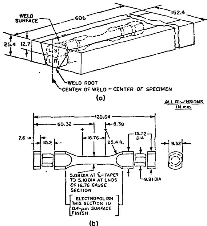
Fig. 3 -- Type 16-8-2 Stainless Steel ASA Weld-metal Test Specimens.
