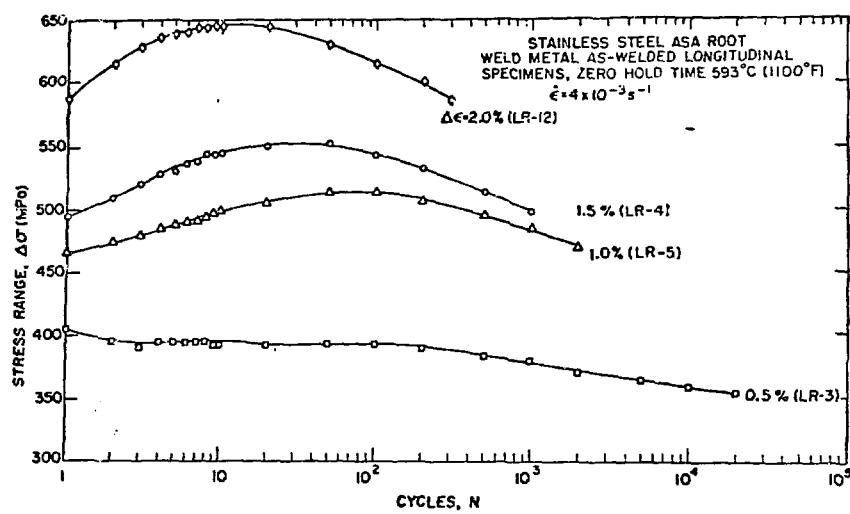
Fig. 7 -- Changes in Stress Range during Reversed Strain Cycling for Root Weld Metal (Specimen Numbers in Parentheses). MSD-63950.
